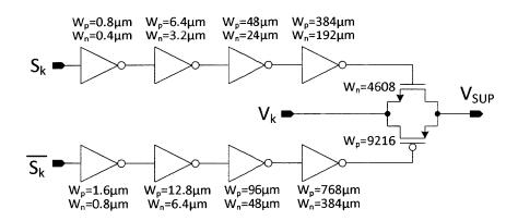
Figure 5-12: Transistor sizes for the power supply switches and the inverter chains used to drive them for the 2.4-GHz AMO IC prototype. The channel length of all the transistors is 0.28  $\mu$ m.
