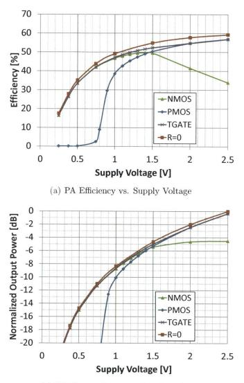
(b) PA Output Power vs. Supply Voltage
