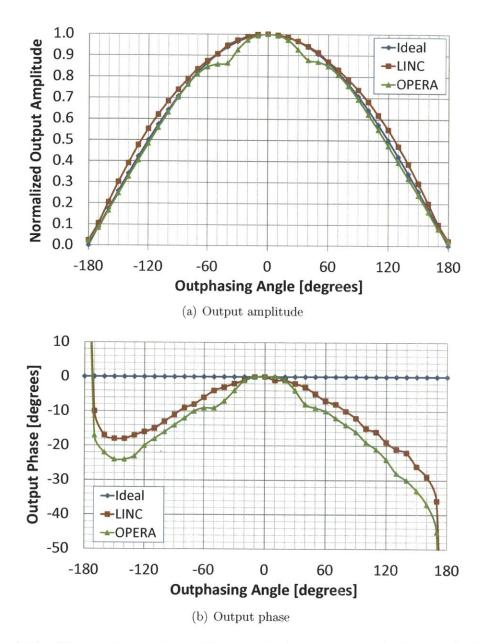
Figure 3-20: Measured output amplitude and phase vs. outphasing angle for the OPERA prototype, with and without energy recovery. (a) Output amplitude. (b) Output phase.
