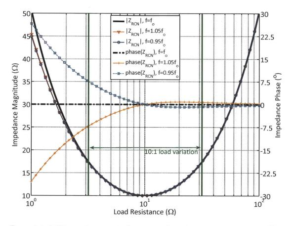
Figure 3-6: RCN impedance vs. load resistance for a frequency deviation of  $\pm 5\%$  of the center operating frequency.  $Z_o = X = 10\Omega$ .
