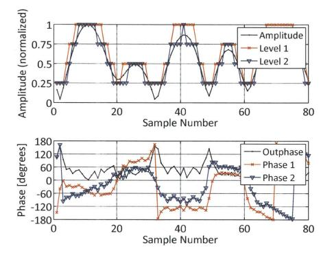
Figure 4-19: Time-domain waveforms of the PA amplitudes and phases resulting from the AMO signal decomposition with DPD,  $A_1$ ,  $A_2$ ,  $\phi_1$ ,  $\phi_1$ , for a segment of the 16-QAM signal shown in Figure 4-18(a), using the example measured data shown in Figure 4-15. The amplitude of the input signal and the outphasing angle between the two PAs is also shown.
