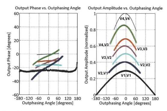
Figure 4-15: Example measurement data for the output amplitude and phase vs. outphasing angle for a real AMO system, which capture the static nonlinearities of the AMO system. Each curve corresponds to a different combination of amplitude levels for the two outphased PAs.
