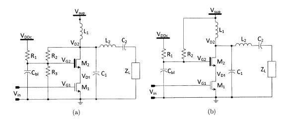
Figure 5-3: (a) Self-biasing topology for a cascode class-E PA used in [60, 61]. (b) Improved self-biasing topology used in this work.
