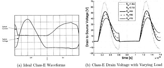
Figure 3-3: (a) Ideal voltage and current waveforms of the main transistor in a class-E PA. (b) The drain voltage waveform of a class-E PA for various values of load resistance.
