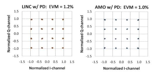
Figure 4-26: Measured demodulated 16-QAM constellation with 6.5-dB PAPR and 50-kHz bandwidth. The EVM is also shown.
