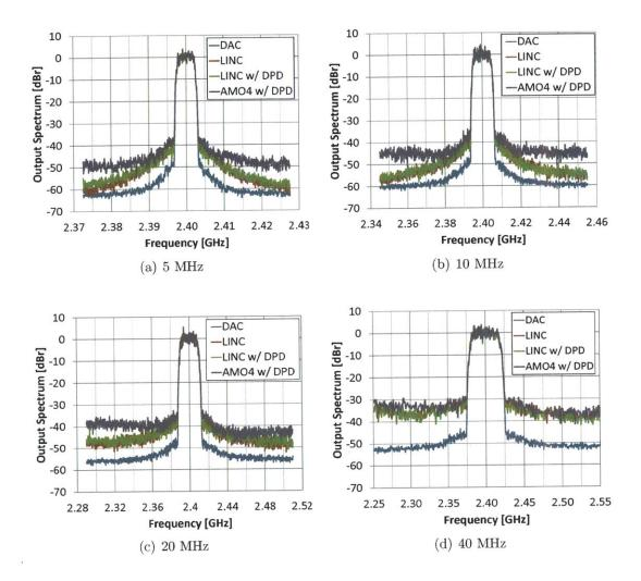
Figure 5-31: Transmit spectrum of a 64-QAM signal at various symbol rates for the 2.4-GHz AMO transmitter. (a) 5 MHz. (b) 10 MHz. (c) 20 MHz. (d) 40 MHz.
