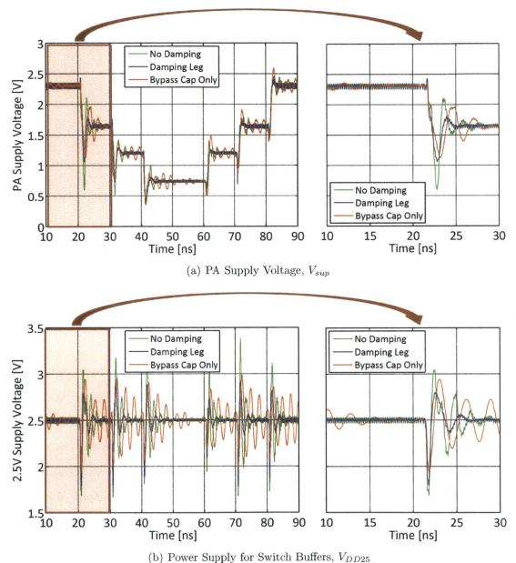
Figure 5-17: Transient ringing for PA supply voltage,  $V_{sup}$  (a) and power supply for switch buffers,  $V_{DD25}$  (b) in the 2.4-GHz AMO IC prototype.
