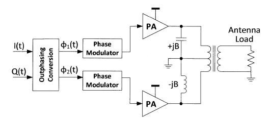
Figure 2-9: Chireix outphasing transmitter.
