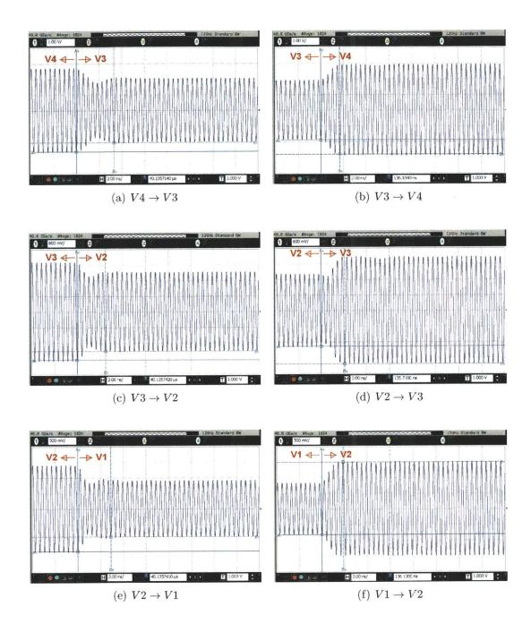
Figure 5-25: Measured step response of the 2.4-GHz AMO transmitter output envelope when the supply voltage is changed for both PAs. (a)  $V4 \rightarrow V3$ . (b)  $V3 \rightarrow V4$ . (c)  $V3 \rightarrow V2$ . (d)  $V2 \rightarrow V3$ . (e)  $V2 \rightarrow V1$ . (f)  $V1 \rightarrow V2$ .
