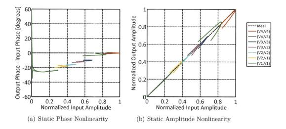
Figure 4-16: Amplitude and phase linearity plots for the example measurement data given in Figure 4-15. (a) Difference between the measured output phase and the ideal input phase, plotted vs. the ideal input amplitude. (b) Measured output amplitude vs. the ideal input amplitude. The ideal input amplitudes and phases are the result from the ideal AMO signal decomposition given in Section 4.2.
