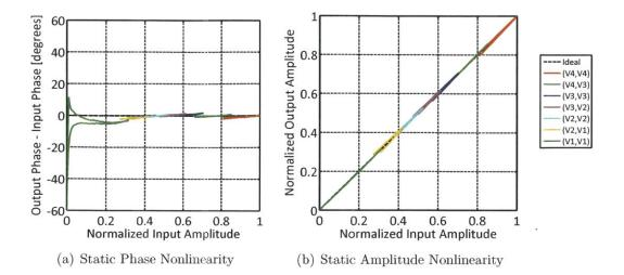
Figure 5-24: Amplitude and phase linearity plots for the measurement data given in Figure 5-23. (a) Difference between the measured output phase and the ideal input phase, plotted vs. the ideal input amplitude. (b) Measured output amplitude vs. the ideal input amplitude. The ideal input amplitudes and phases are the result from the ideal AMO signal decomposition given in Section 4.2.
