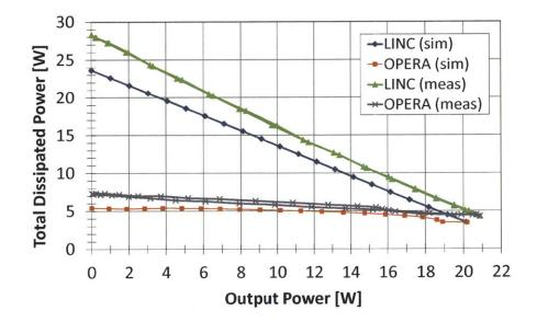
Figure 3-19: Total dissipated power vs. output power in the OPERA prototype with and without energy recovery.
