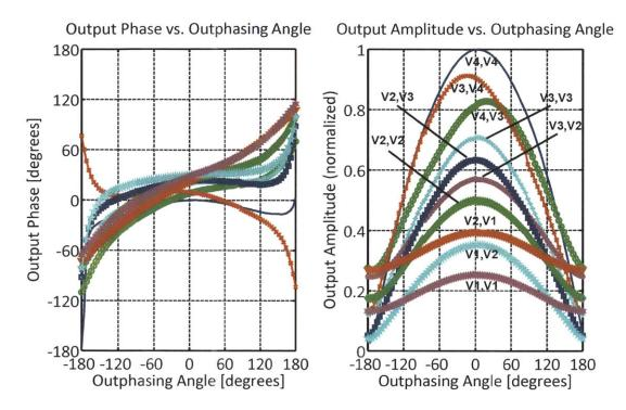
Figure 4-23: Measured output amplitude and phase vs. outphasing angle for the prototype AMO system with DPWM. Each curve corresponds to a different combination of discrete pulse widths for the two outphased PAs.
