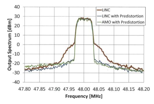
Figure 4-27: Measured transmit spectrum of the 50-kHz, 16-QAM signal for both the LINC and AMO-DPWM systems.
