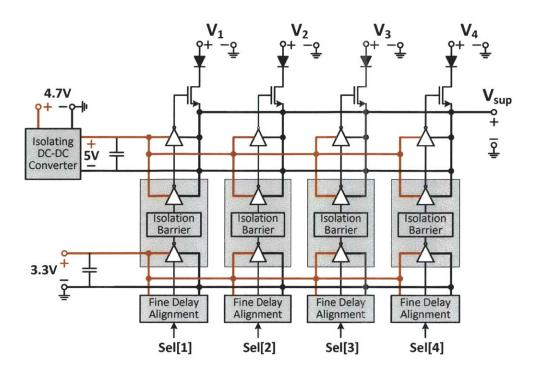
Figure 4-36: 4-level discrete supply modulator for the 1.95-GHz AMO prototype.
