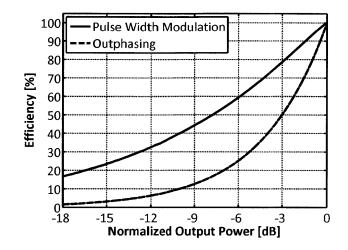
Figure 2-7: Comparison between the power efficiency of outphasing and pulse-width modulation depending on output power.
