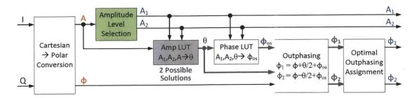
Figure 4-17: Block diagram for the AMO signal decomposition with DPD based on lookup tables.
