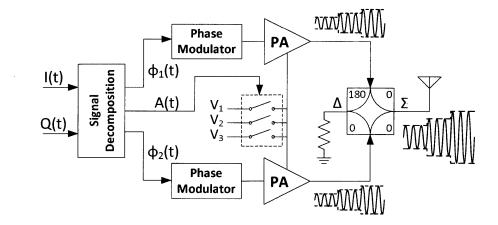
Figure 2-11: Multi-level LINC architecture. Three supply voltages are shown in the figure, but there can be any number of supply voltages greater than 1 for the ML-LINC system.
