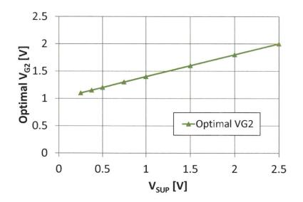
Figure 5-5: Optimal  $V_{G2}$  vs.  $V_{sup}$  for maximum efficiency from simulation of the cascode class-E PA for the 2.4-GHz AMO IC prototype.
