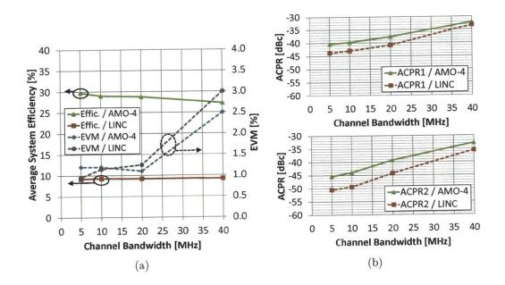
Figure 5-29: Performance comparison of the LINC and 4-level AMO systems for the 2.4-GHz AMO IC prototype, for the transmission of a 7.0-dB PAPR 64-QAM signal at various channel bandwidths. (a) EVM and average system efficiency. (b) ACPR at 1st and 2nd channel offsets.
