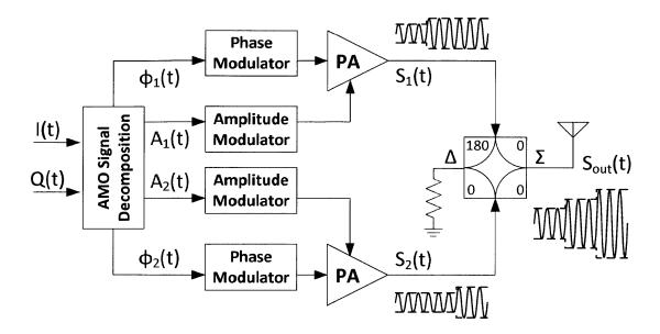
Figure 4-1: Asymmetric multilevel outphasing (AMO) architecture.
