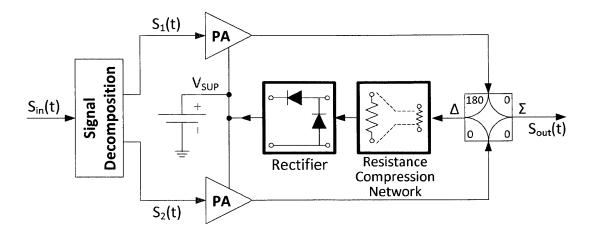
Figure 1-4: Outphasing energy recovery amplifier, utilizing a resistance compression network in the power recycling network.
