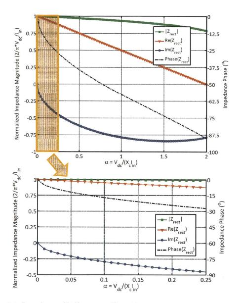
Figure 3-8: Impedance of half-wave rectifier with parasitic capacitance vs. parameter  $\alpha = V_{dc}/(X_c I_{in})$ . As  $\alpha$  increases, the impedance looks increasingly capacitive.
