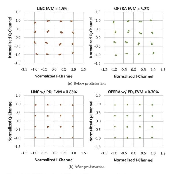
Figure 3-23: EVM for the 50-kHz 16-QAM transmission for the OPERA prototype with and without energy recovery. (a) Before predistortion. (b) After predistortion.
