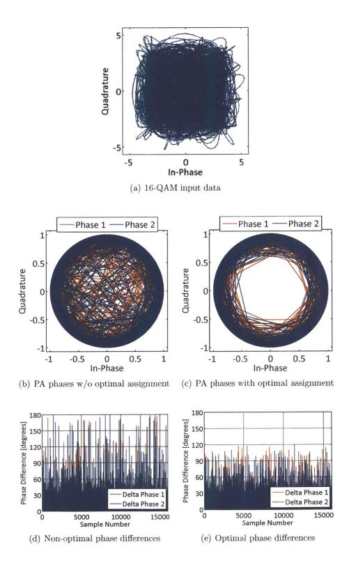
Figure 4-18: The PA phases and phase differences after the AMO signal decomposition with and without the optimal outphasing assignment.
