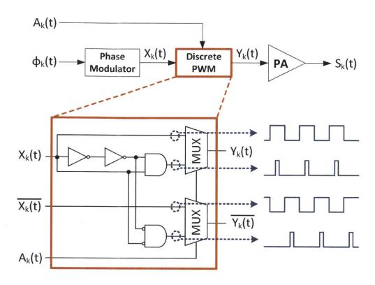
Figure 4-10: Example implementation of a 2-level discrete pulse-width modulator (DPWM).
