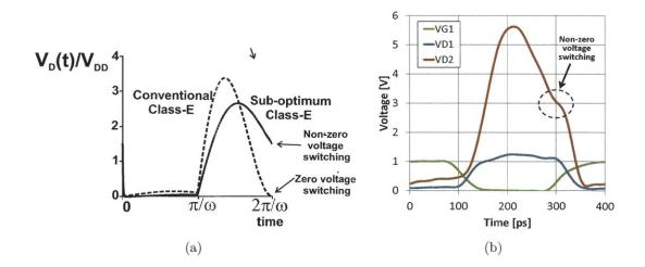
Figure 5-2: (a) Drain voltage waveforms for the conventional class-E PA and variable-voltage class-E PA. (b) Simulated drain voltage waveform for the PA used in the 2.4-GHz AMO IC prototype.
