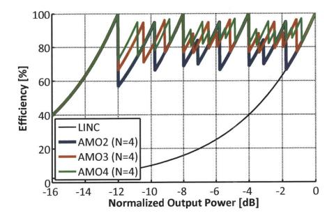
Figure 6-2: Theoretical efficiency for the AMO system using 2, 3, and 4 PAs. 4 supply voltages are available for each case, with the amplitude levels spaced 4 dB apart.
