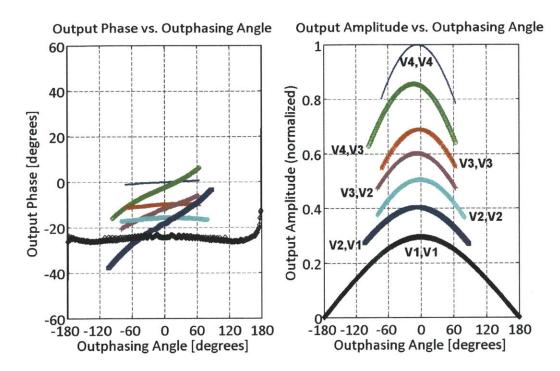
Figure 4-39: Measured static output amplitude and phase vs. outphasing angle for the 1.95-GHz AMO transmitter. Each curve corresponds to a different combination of supply voltages for the two outphased PAs.
