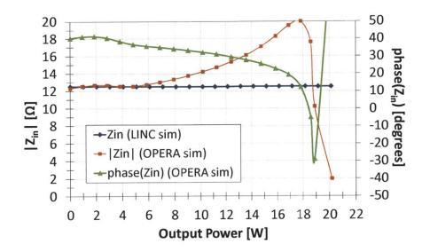
Figure 3-15: Simulated isolation port impedance vs. output power in the OPERA prototype. The desired isolation port impedance is also shown for reference.
