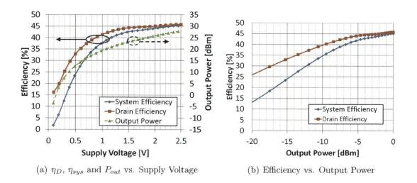
Figure 5-21: (a) Measured drain efficiency, system efficiency, and output power vs. supply voltage for the AMO IC prototype at 2.4 GHz. (b) Measured efficiency vs. output power.
