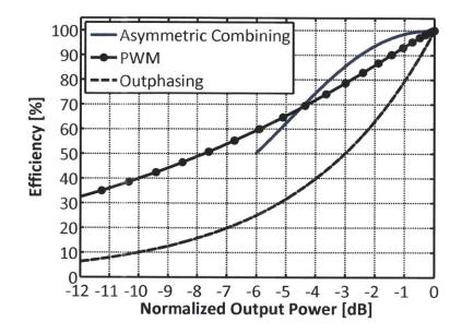
Figure 4-5: Asymmetric 2-way power combining efficiency vs. output power, for the special case where  $\phi_1 = \phi_2$  and the amplitude of  $A_2$  is swept continuously between 0 and  $A_1$ . The efficiency of outphasing and class-E PWM (described in Section 2.3) is also shown for comparison.
