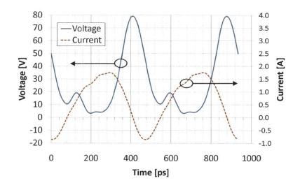
Figure 4-31: Simulated drain voltage and current for the class-E GaN PA after deembedding package parasitics, indicating class-E operation. The design frequency was 2.14 GHz.
