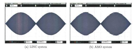
Figure 5-27: Measured output waveform of the IC prototype for a 1-MHz baseband sine wave transmission. The sampling rate of the digital data is 200 MHz and the RF carrier frequency is 2.4 GHz. (a) LINC system. (b) AMO system.
