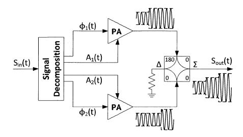
Figure 1-5: Asymmetric multilevel outphasing (AMO) architecture.
