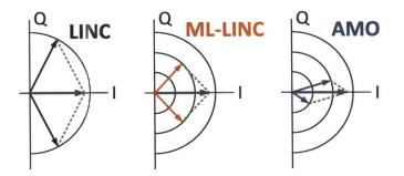
Figure 4-2: Signal component vector diagram for LINC, ML-LINC, and AMO. The smallest outphasing angle is achieved with AMO.
