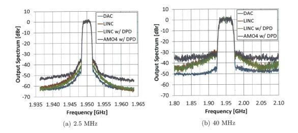
Figure 4-46: Transmit spectrum of a 16-QAM signal at 2.5 MHz and 40 MHz symbol rate for the 1.95-GHz AMO transmitter. (a) 2.5 MHz. (b) 40 MHz.
