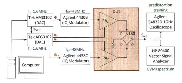
Figure 4-25: Outphasing system testbench for 50-kHz 16-QAM transmission at a carrier frequency of 48 MHz.
