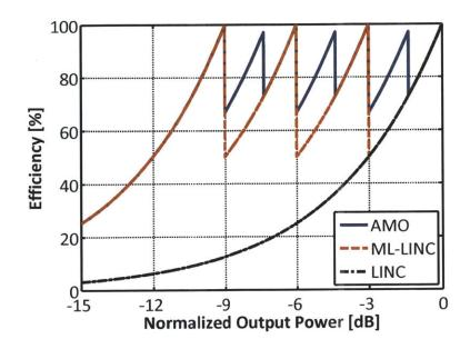
Figure 4-6: Efficiency vs. output power of AMO modulation compared to LINC and ML-LINC when 4 different PA amplitude levels are available, assuming 100% efficiency in the PAs.
