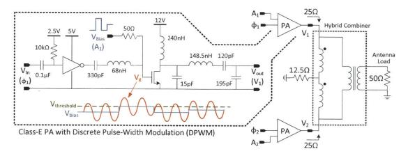
Figure 4-21: Prototype 48-MHz AMO transmitter with DPWM.
