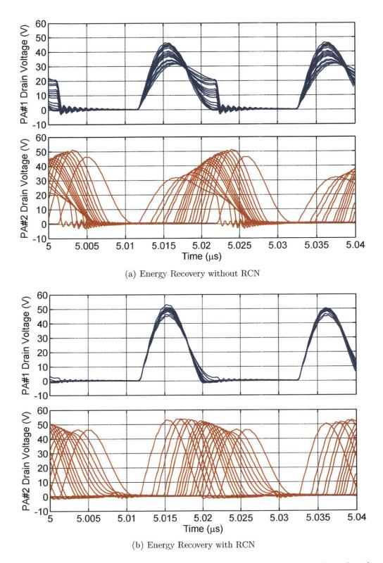
Figure 3-16: Simulated PA drain voltages in the OPERA prototype with and without the resistance compression network, for various outphasing angles and output powers.
