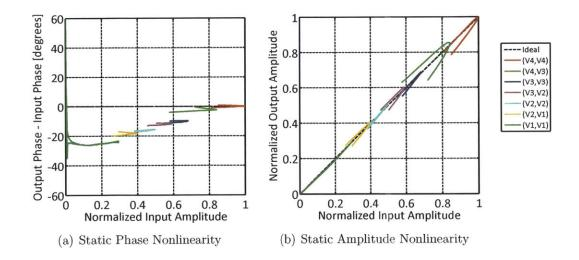
Figure 4-40: Amplitude and phase linearity plots for the measurement data given in Figure 4-39. (a) Difference between the measured output phase and the ideal input phase, plotted vs. the ideal input amplitude. (b) Measured output amplitude vs. the ideal input amplitude. The ideal input amplitudes and phases are the result from the ideal AMO signal decomposition given in Section 4.2.
