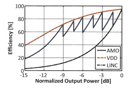
Figure 4-9: Efficiency vs. output power of the AMO system with DSVM when 4 different supply voltage levels are available, assuming a fixed power loss of -13dB relative to the maximum output power. The only other loss accounted for in the plot is the loss due to the asymmetric combining.
