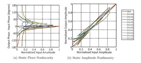
Figure 4-24: Amplitude and phase linearity plots for the measurement data given in Figure 4-23. (a) Difference between the measured output phase and the ideal input phase, plotted vs. the ideal input amplitude. (b) Measured output amplitude vs. the ideal input amplitude. The ideal input amplitudes and phases are the result from the ideal AMO signal decomposition given in Section 4.2.
