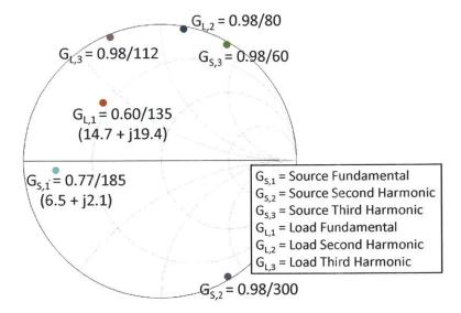
Figure 4-30: Optimum input and output impedances at the fundamental, 2nd harmonic, and 3rd harmonic of the RF carrier frequency for maximum efficiency for the class-E GaN PA.
