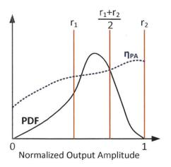
Figure 4-13: Example amplitude PDF for a signal (black line), along with an example PA efficiency curve  $\eta_{PA}$  vs. output amplitude (blue line). The  $r_k$  are the maximum output amplitudes for each of the different supply voltage levels  $V_{sup,k}$  when both PAs are driven by the same supply. There are 2 amplitude levels available in the example above.
