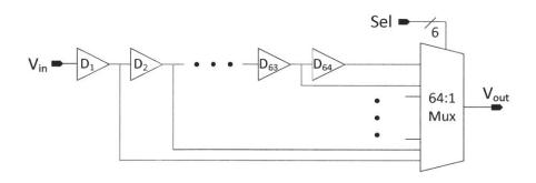
Figure 5-11: Block diagram of the delay line used in the delay adjustment circuit and to implement time alignment between the amplitude and phase paths for the 2.4-GHz AMO IC prototype.
