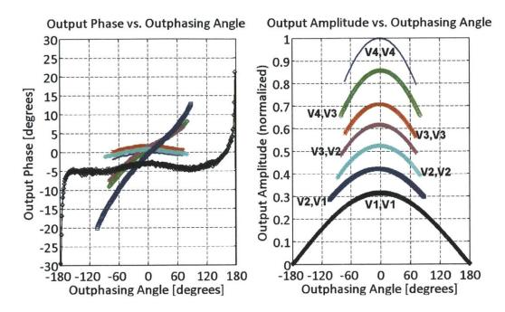
Figure 5-23: Measured static output amplitude and phase vs. outphasing angle for the 2.4-GHz AMO transmitter. Each curve corresponds to a different combination of supply voltages for the two outphased PAs.
