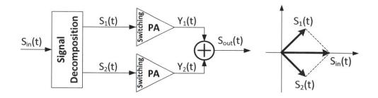
Figure 1-2: (a) LINC principle diagram. (b) LINC vector diagram.
