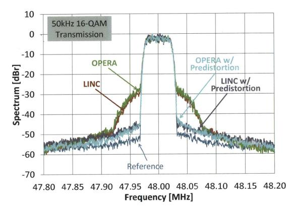
Figure 3-22: Measured output spectrum for 50-kHz 16-QAM transmission with 6.5-dB PAPR, with and without energy recovery, and before and after predistortion. The reference spectrum is the result using only the combiner with a fixed isolation port resistance.
