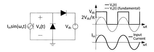
Figure 3-2: Ideal half-wave rectifier with constant voltage load and driven by a sinusoidal current source, along with characteristic waveforms. The input current and the fundamental of the input voltage are in phase.
