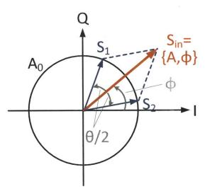
Figure 2-2: LINC vector diagram, including notational convention.
