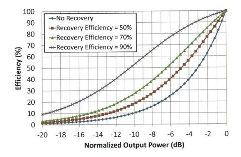
Figure 3-9: Theoretical OPERA efficiency as a function of normalized output power, showing the effect of the energy recovery network efficiency. The PAs are assumed to be 100% efficient, with no insertion loss in the power combiner.
