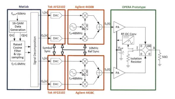
Figure 3-21: Outphasing system testbench used for the 48-MHz OPERA prototype for 50-kHz 16-QAM transmission.
