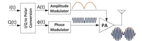
Figure 2-4: Conventional polar architecture.
