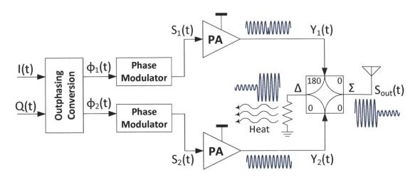
Figure 2-1: Conventional outphasing, or LINC, architecture.
