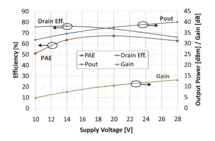
Figure 4-35: Measured PAE, drain efficiency, output power, and gain of the class-E GaN PA at 1.95 GHz.
