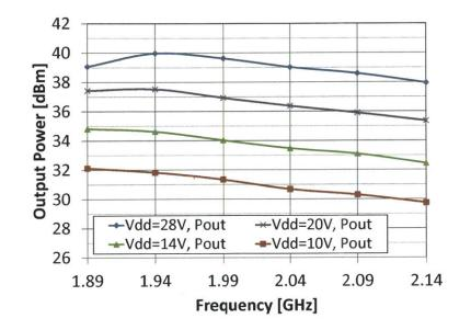
Figure 4-33: Measured output power vs. frequency at various supply voltages for the class-E GaN PA.
