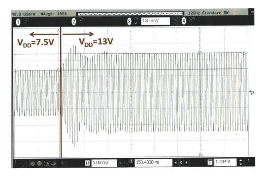
Figure 4-41: Measured step response of the 1.95-GHz AMO transmitter output envelope when the supply voltage is changed from 7.5 V to 13 V.
