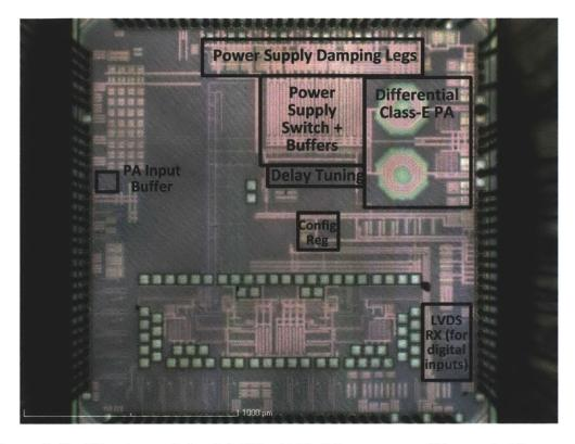
Figure 5-18: Die photo of the 2.4-GHz AMO IC prototype. The total chip area is  $2x2 \text{ mm}^2$ . Each chip has one PA and one discrete supply voltage modulator.
