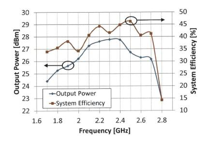
Figure 5-20: Measured output power and system efficiency vs. frequency for the AMO IC prototype.
