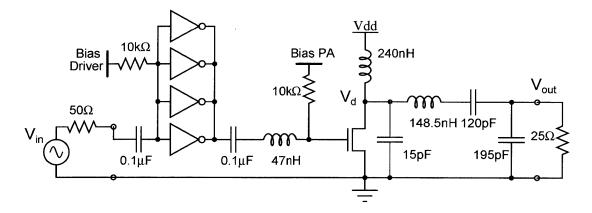
Figure 3-13: Circuit schematic of the class-E power amplifier used in the OPERA prototype.
