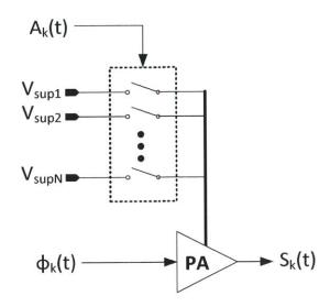
Figure 4-8: Example of a discrete supply-voltage modulator (DSVM).
