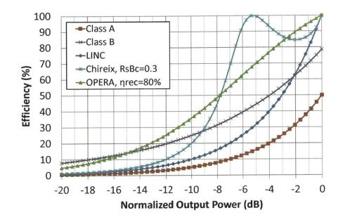
Figure 3-11: Comparison of theoretical OPERA efficiency to that of other PA architectures. Note that the Chireix efficiency curve does not reflect the efficiency degradation that will occur due to the widely varying impedance presented to the outphased PAs as the output power varies.
