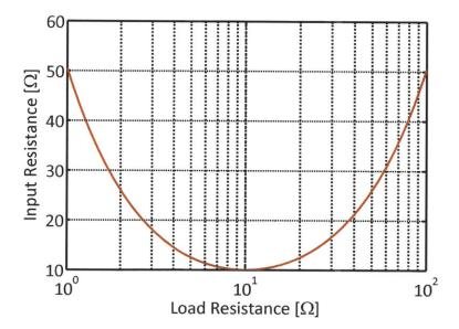
Figure 3-5: Input resistance  $R_{RCN}$  of the RCN shown in Figure 3-4 vs. load resistance  $R_{rect}$  for  $X = 10\Omega$ .
