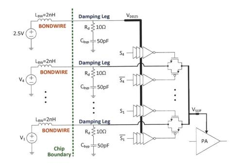
Figure 5-16: Discrete supply voltage modulator with damping legs to reduce the transient ringing on the on-chip supply voltage nodes in the 2.4-GHz AMO IC prototype.
