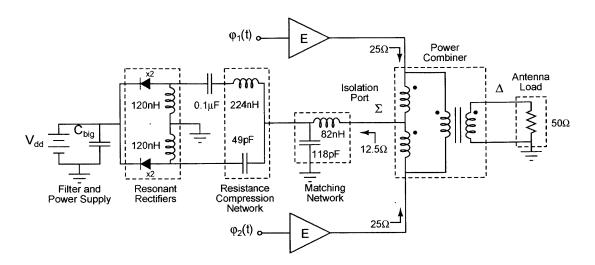
Figure 3-12: Prototype OPERA system with resistance-compressed rectifier for energy recovery. Each rectifier branch is implemented with a pair of paralleled SS16 Schottky diodes. The impedance at each port of the power combiner that is required for matching and isolation is also indicated.
