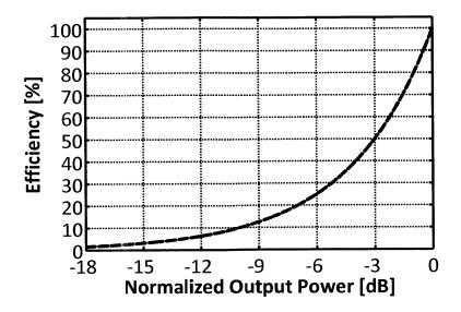
Figure 2-3: Efficiency vs. output power for the outphasing system using a conventional isolating combiner.
