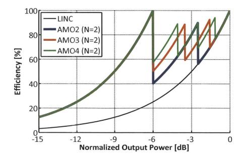
Figure 6-1: Theoretical efficiency for the AMO system using 2, 3, and 4 PAs. 2 supply voltages are available for each case, with the amplitude levels spaced 6 dB apart.
