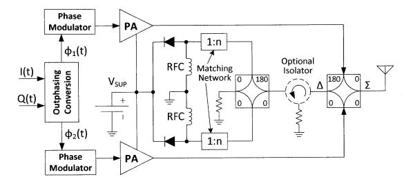
Figure 2-10: Outphasing power amplifier with power recycling network.
