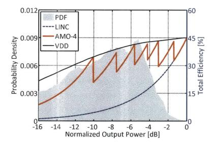
Figure 5-22: Measured efficiency vs. output power for the 2.4-GHz AMO IC prototype, along with the optimized amplitude levels for a 64-QAM signal with 7.0-dB PAPR. The PDF of the 64-QAM signal is also shown.
