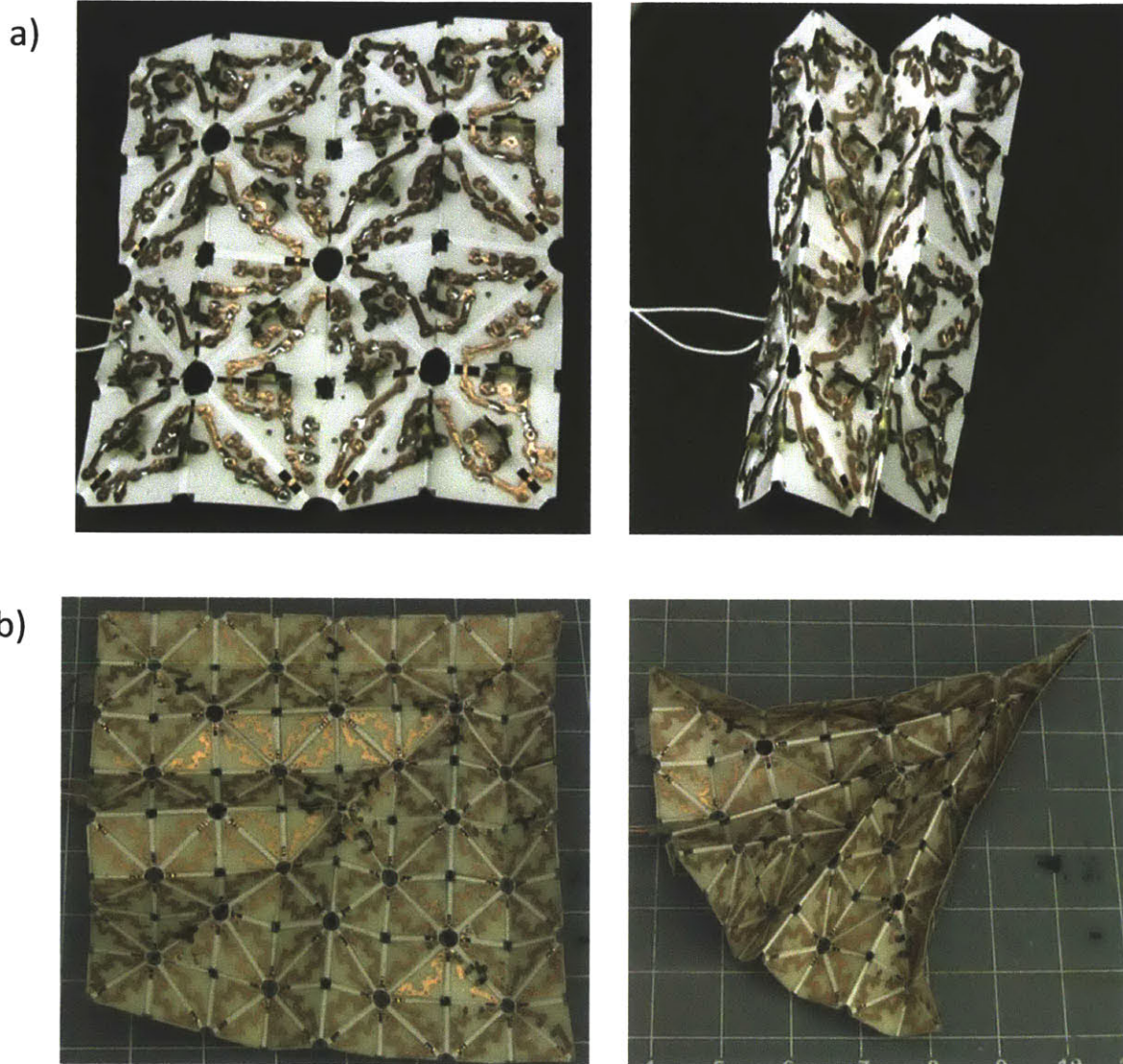
Figure 4-1: Two examples of different implementations of self-folding sheets (Ch. 6). (a) 4 \times 4 self-folding sheet with the vertical folding program. The sheet is of size 96mm \times 96mm and uses copper tape. (b) 8 \times 8 self-folding sheet with the space shuttle-like shape folding program. The sheet is of size 192mm \times 192mm and uses copper foil and PEEK. Each device was created using the same architecture but a different manufacturing process
