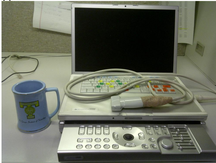
Figure 2-4. Laptop based portable ultrasound system. Coffee mug shown for scale.
