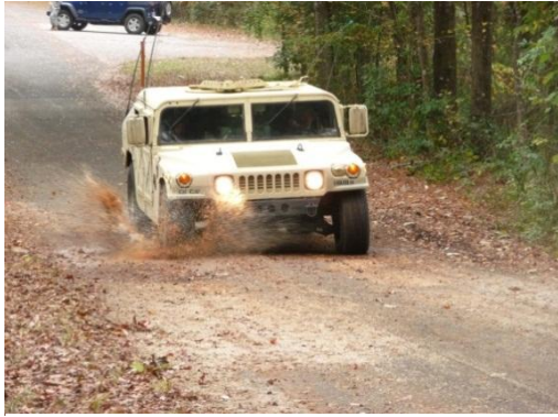
Figure 6-3. Humvee used in Trial at Ft. Rucker hitting Pothole
