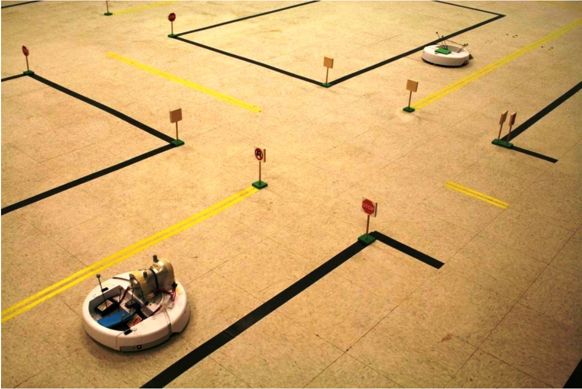
Figure 4-2: The road network used for experiments. In this image, both a human-driven vehicle (front-left) and autonomous vehicle (back-right) are approaching a four-way, stop-sign intersection.
