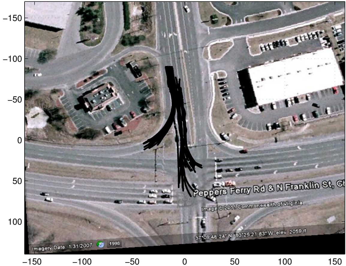
Figure 3-10: Satellite image of the Peppers Ferry intersection adapted from Google Earth. CICAS-V trajectories of vehicles at Pepper’s Ferry intersection were used to test the algorithms presented in this section. 45 instances are shown as black lines superimposed on the intersection image.
