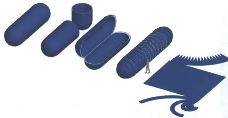
Possible reconfigurations of a 10,000 gallon steel tank.
