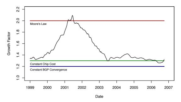
Figure 1-2: Normalized growth factor (smoothed over a 2 year window) of the Internet routing table relative to Moore's Law and other desirable engineering objectives, semiconductor chip cost and routing protocol convergence time, from 1999-2007 [Li06].
