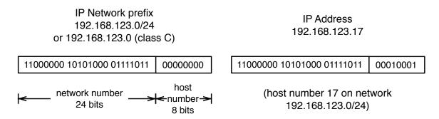
Figure 2-3: An example of an IP network prefix and full IP address, illustrating the distinction between the network number and host number components of the address. Note that the prefix length (e.g. /24) indicates the position of the partition between the network number and the host number, and thus the number of bits allocated to each.
