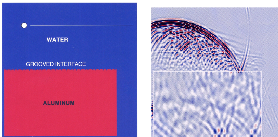
Figure 2 A schematic of the laboratory model used by Schultz and Toksöz (1995) to study scattering from an aluminum block with parallel grooves cut into the surface (left panel). The right panel shows a wavefield snapshot from a finite difference model of the aluminum block. Note the scattered wave energy that follows the reflection from the top of the block.
