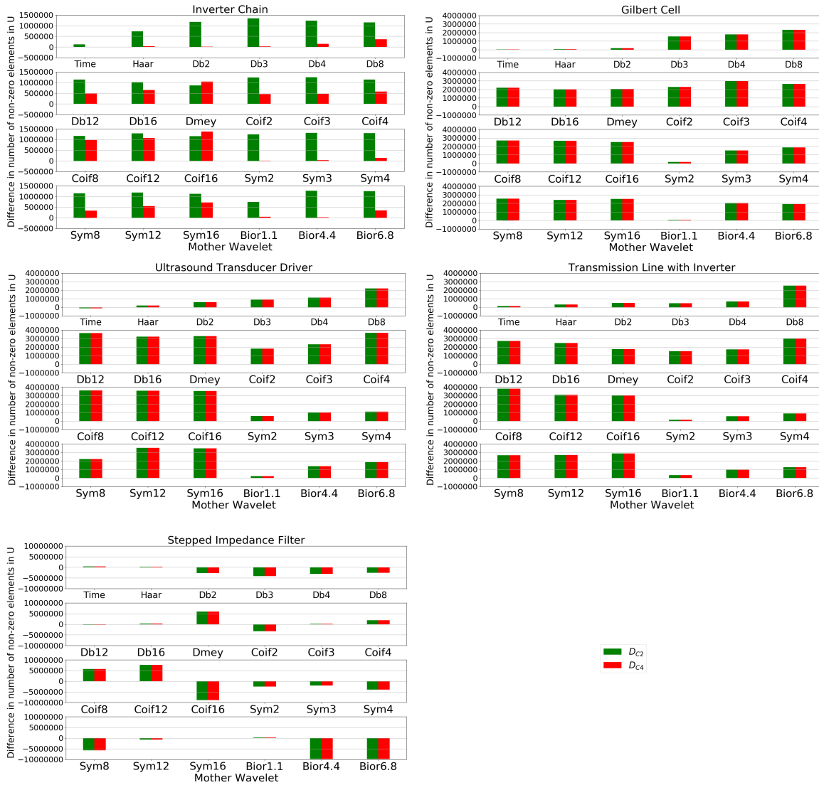
Figure 4.34: Difference between the average density of the U matrices with and without adaptive Jacobian matrix thresholding. A positive number indicates that the U matrices resulting from the non-thresholded Jacobian matrices have a higher number of non-zero elements, on average, than the U matrices resulting from the adaptively thresholded Jacobian matrices.
