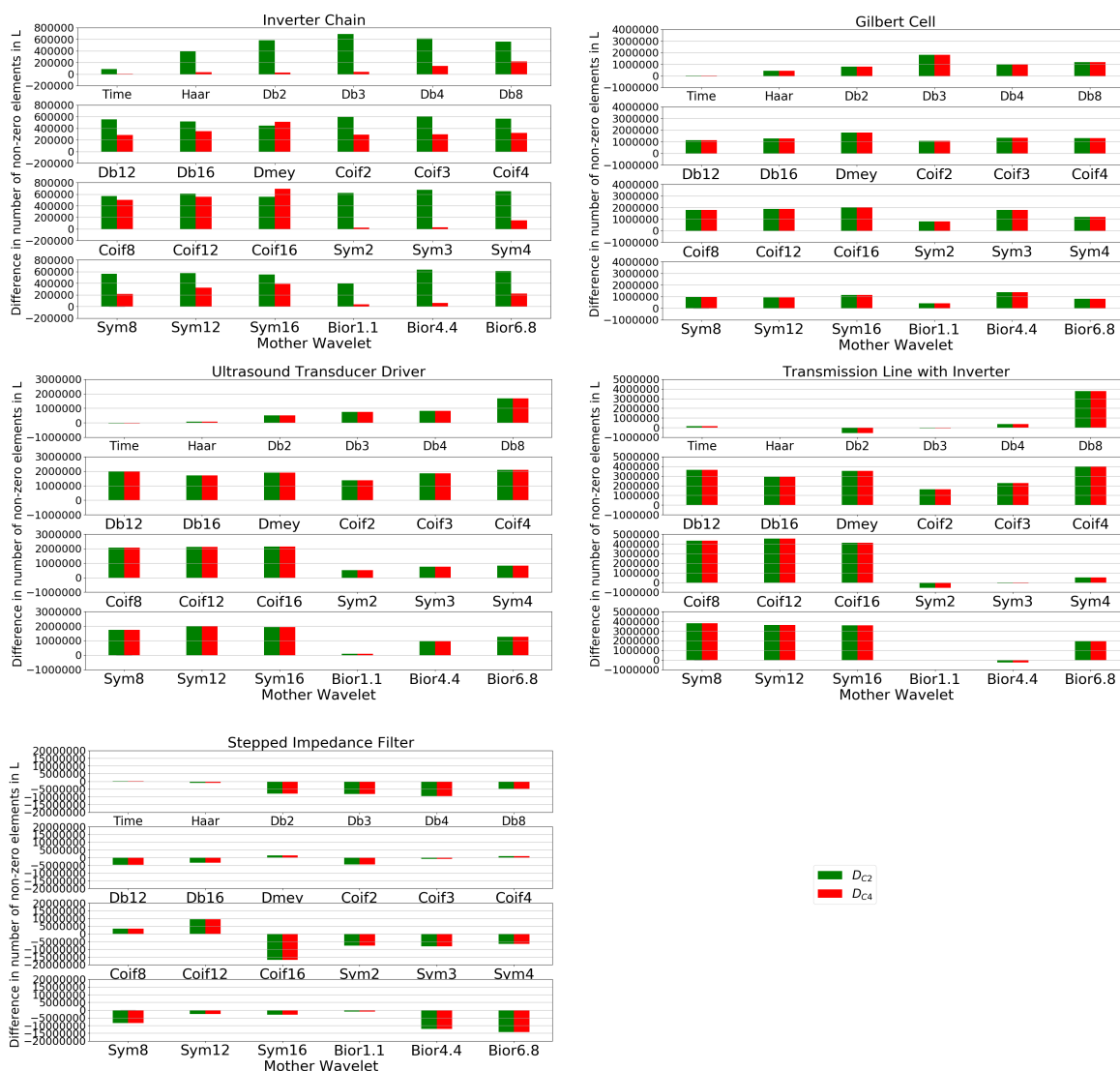
Figure 4.33: Difference between the average density of the L matrices with and without adaptive Jacobian matrix thresholding. A positive number indicates that the L matrices resulting from the non-thresholded Jacobian matrices have a higher number of non-zero elements, on average, than the L matrices resulting from the adaptively thresholded Jacobian matrices.
