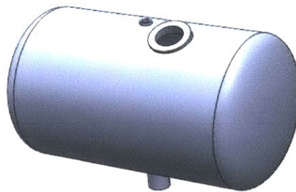
Figure 11: Aft Ballast Tank
