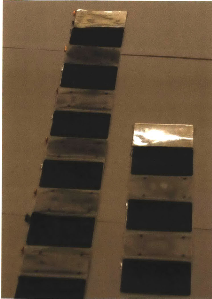
Figure 16 Bare Pouch Cell Unrolled, Showing Alternating Layers of Anode and Cathode Plates Adhered to Separator
