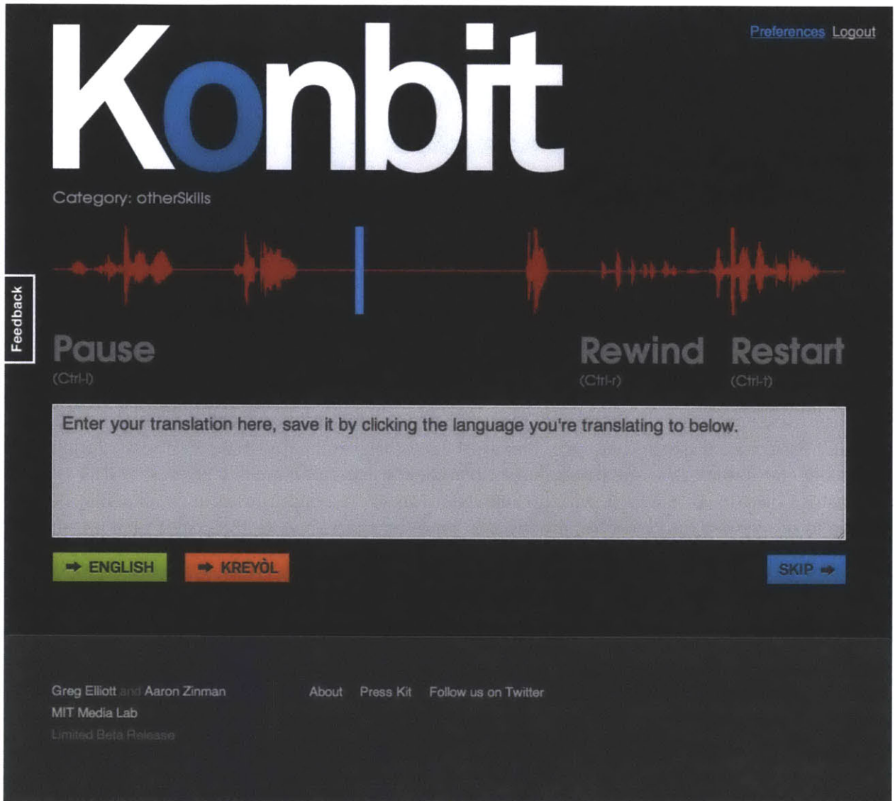
Figure 1 - the main translation interface, which consists of an audio file and its accompanying waveform, controls for the audio player, a text box for entering the translation, and buttons for each language the translator spoke
