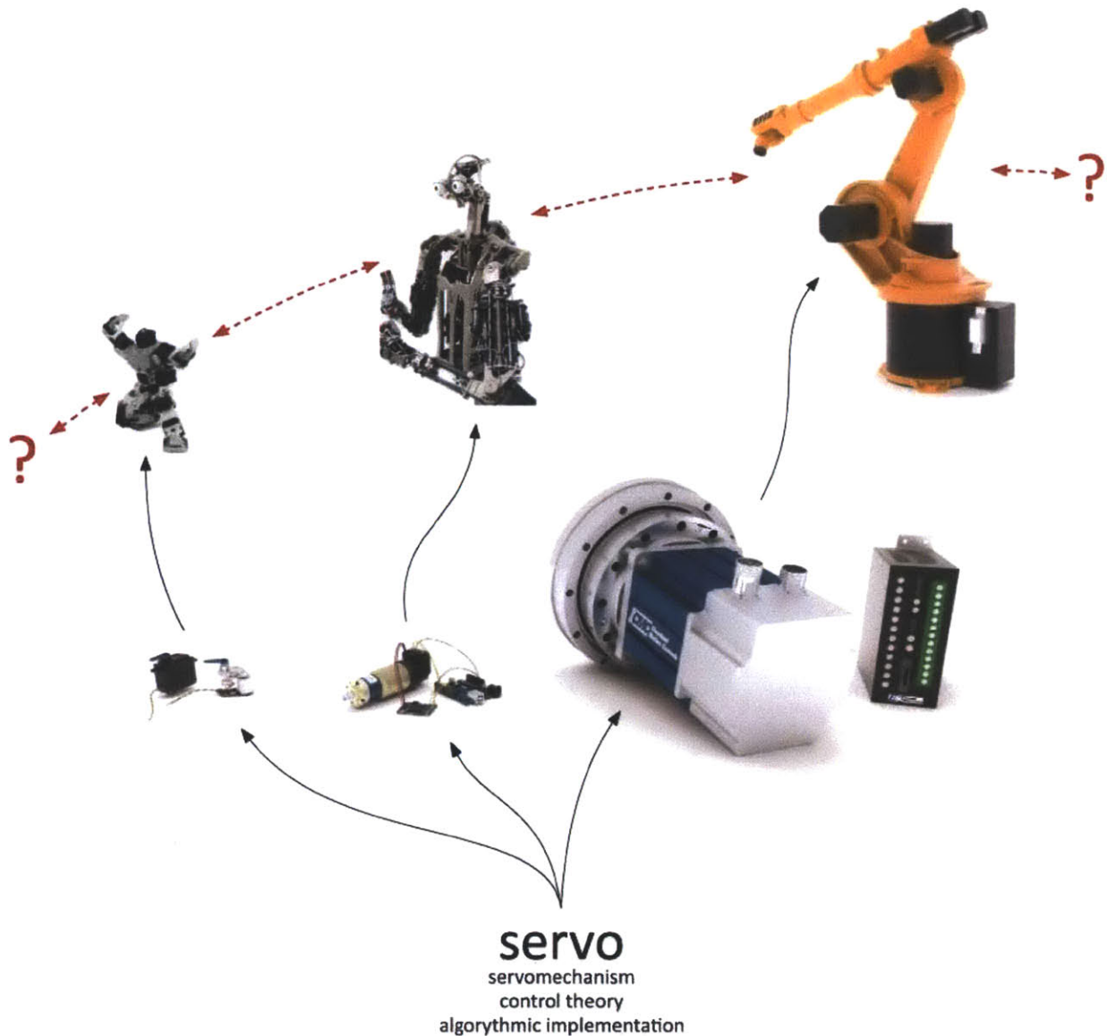
Figure 2.14 (Above) Diagram of the servo motors and their applications raising the question of moving across scale indicated by the red line. Every iteration involving a change in scale requires going back to the root of the diagram and re-implement the servo at the specific scale
