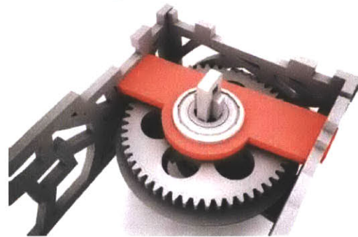
wrong position of ball bearing support ribs!
