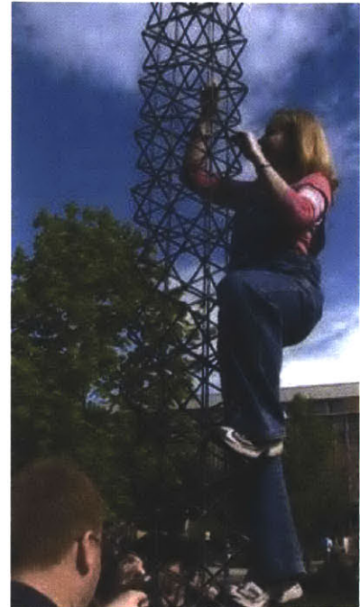
Figure 2.26 (Above) ISO Truss lightweight carbon fiber structure supporting the weight of a person climbing it.
