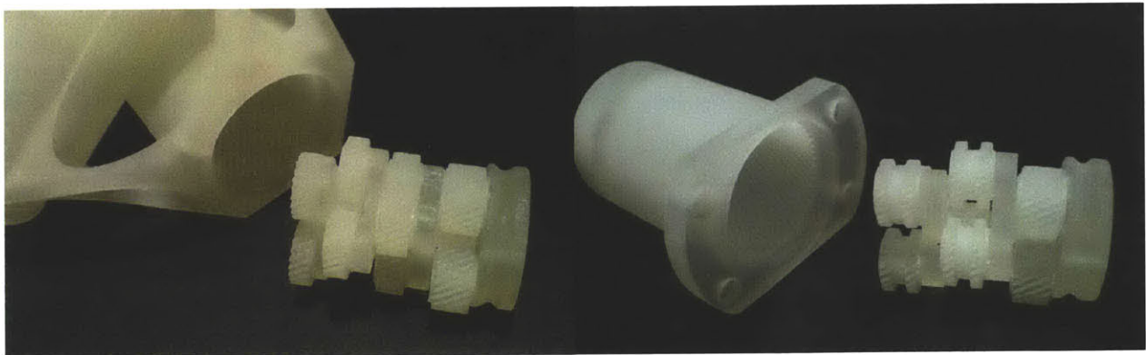
Figure 3.49 (Above) CG rendering of planetary gear box intended for 3D printing and demonstrating a dynamic and form oriented integration of the planetary concept. Photos of two staggered planetary gear boxes with 3 and 4 stages utilizing helical gears.
