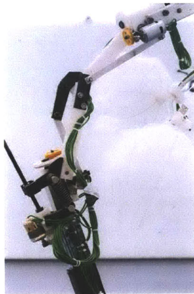
Figure 2.10 (TOP) 003#02 Three kinetic sculptures imitating orchids in motion. Figure 2.11 (Above) 003#02 Detail showing wiring, gears, motors, spring, joints and structure of the machine.
