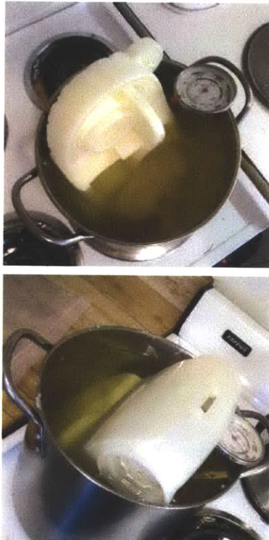
Figure 5.83 (Above) melting and extracting the Invisin PolyJet 3D print in corn oil.
