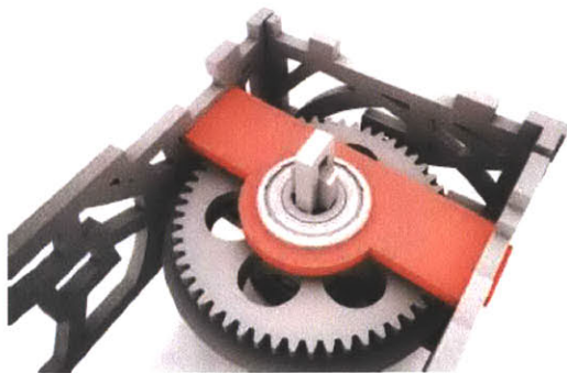
correct position of ball bearing support ribs.
