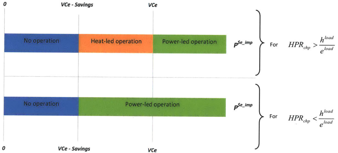
Figure 6.2.25: Micro-CHP operational outputs under different prices & load conditions
