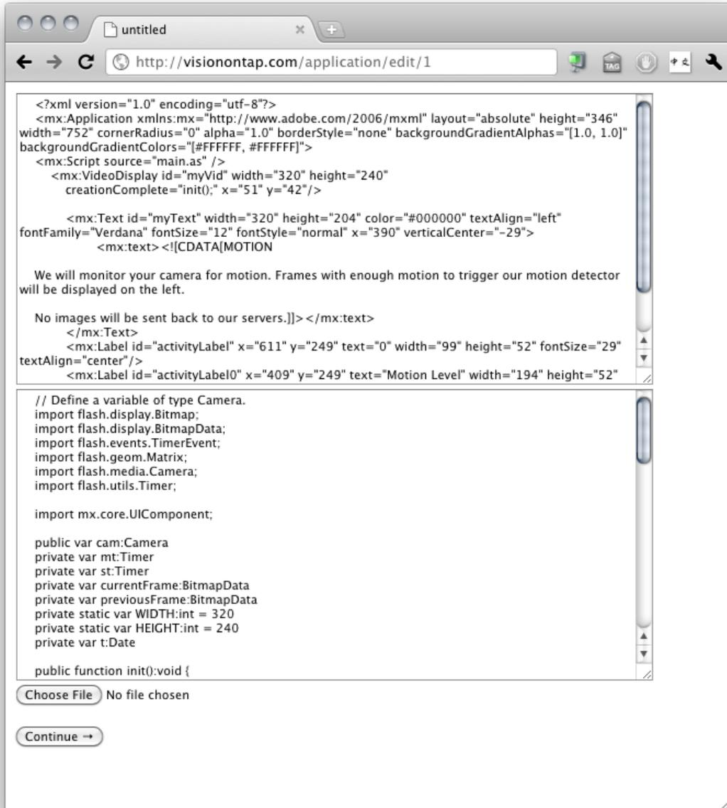
Figure 2-2: The initial creation interface provided by the Vision on Tap system. The author may either edit the code directly in the web form for simple applications or upload the project source in zip format by specifying a file via the file choosing widget. After the form is submitted, the user is provided with the URL for their application.
