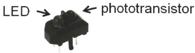
Figure 2.20: Optical position sensor measures reflected light from a surface. The intensity of light is often correlated with the distance of the surface away from the sensor.
