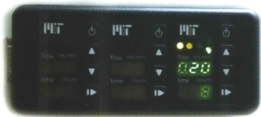
Figure 2.23: Control panel for operating 3 bioreactors.
