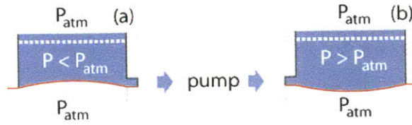
Figure 2.13: A two-capacitor system filters flow pulses both entering (a) and leaving (b) the pump. In (a), lower than atmospheric pressure draws fluid through the fluidic resistor, and in (b) elevated pressures drive flow through the resistor. The bioreactor uses a single capacitor between the pump and scaffold.
