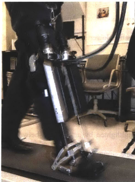
Figure 3-2: An unimpaired human subject wearing Anklebot while walking on a treadmill.
