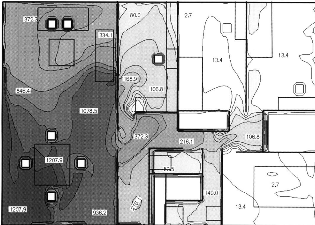
Figure 4.1.1.12 Vapor concentration gradient at the end of dinner with bimodal ventilation showing migration of pollutants only towards rooms with exhausts
