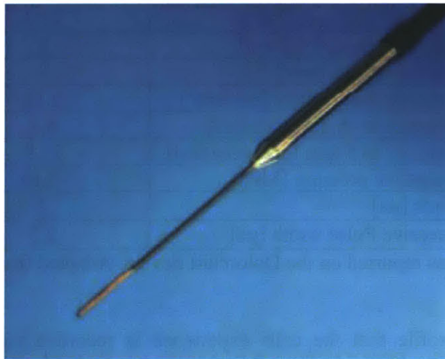
Figure 6-5: Onda HNS needle hydrophone used for measuring pressures in collagen gels. From http://www.ondacorp.com/images/brochures/Onda_HNS_DataSheet.pdf
