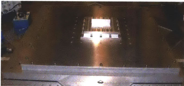
Figure 5-14: Panel with 6in x 6in Box (LT) and Corresponding Frequency Response Plot (RT). FNF = 75 Hz.
