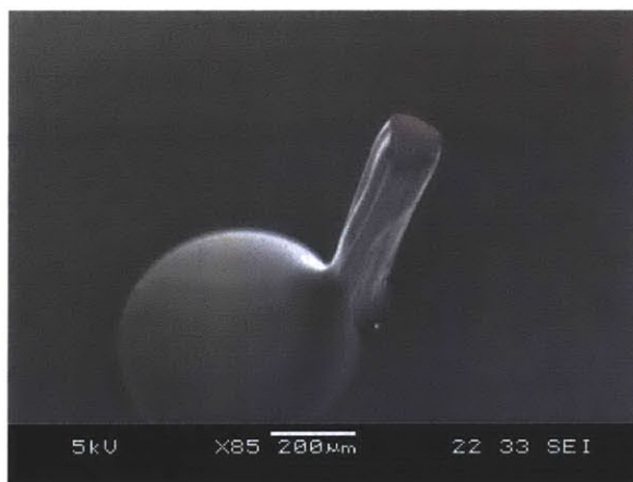
Figure 3-4: SEM image demonstrating wetting of a column of vertically aligned carbon nano-tubes with ionic liquid.
