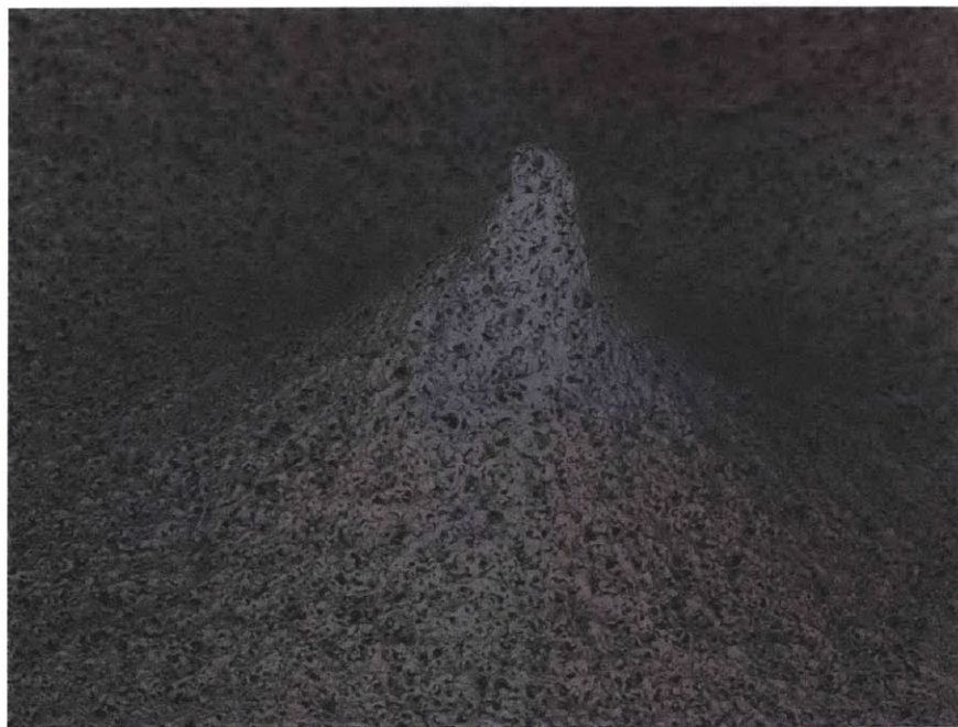
Figure 6-43: SEM images of emitters formed after secondary etching. The structures are generally smooth with no signs of etching within the pores, despite a short etch time.
