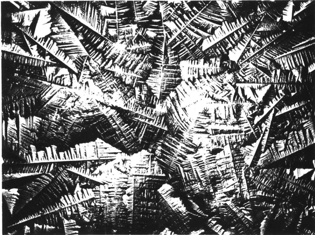
Fig. 15. The surface of an ingot of antimony, showing dendritic crystals which have grown to interference with each other. (This pattern was the mystic Star of Antimony of the alchemists.) About natural size. ( Photo Courtesy The Science Museum, London. Crown copyright )
