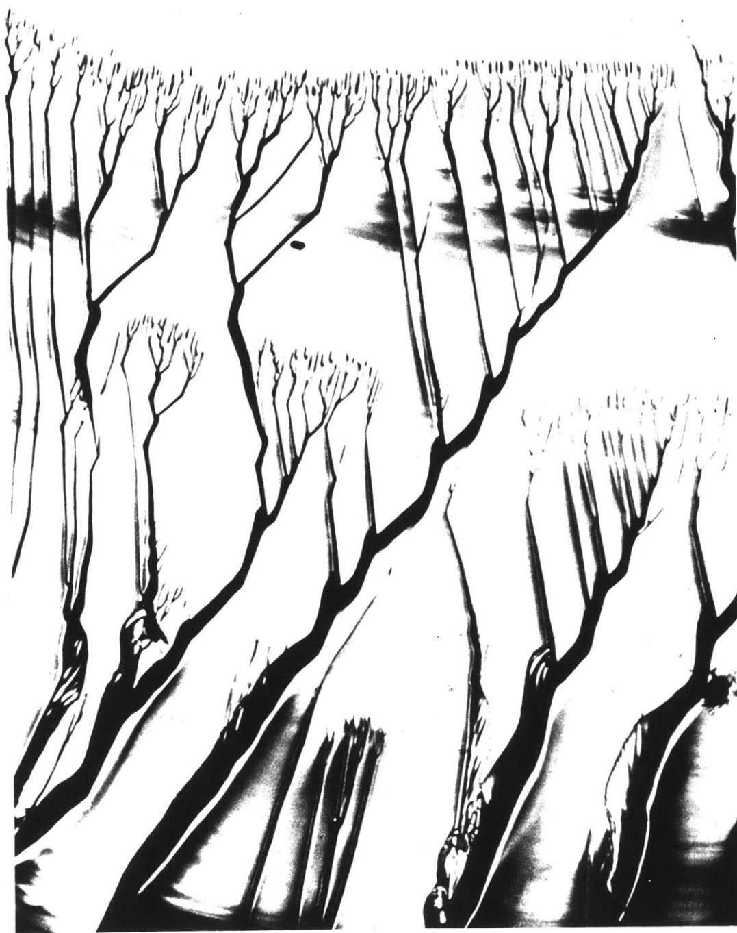
Fig. 16. Pattern of ridges formed by a crack moving in a crystal of a brittle compound of copper and magnesium, \text{Cu}_2\text{Mg} . The crack proceeded from the top to the bottom of the figure. Magnification \times 300 . ( Photo Courtesy Duane Mizer, Dow Metal Products Company )
