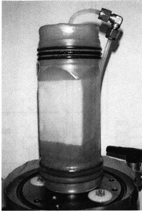
Figure 4-18: Photograph of partial setup of specimen for Flexible Wall Permeameter (cubic specimen)
