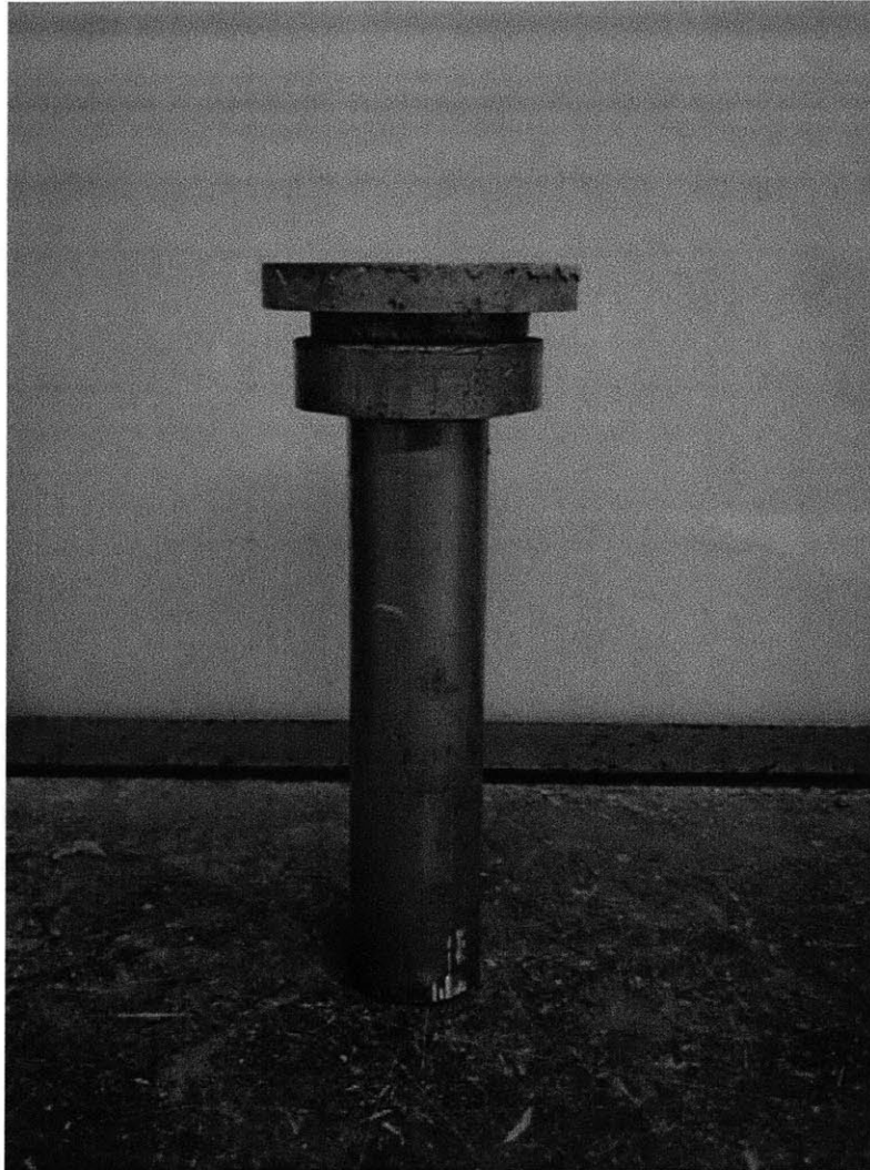
Figure 3-3: Jacking object that can be used to push specimen out of a sample tube. The top of the object is approximately equal to the specimen diameter.
