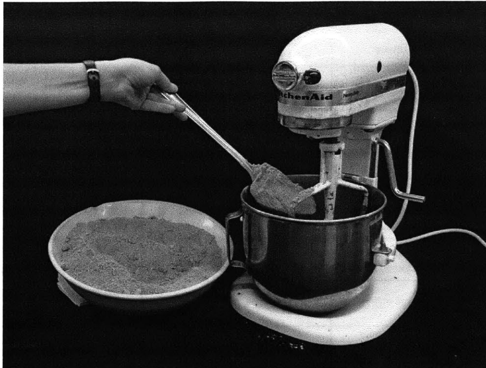
Figure 4-1: Mixing RBBC powder with 16 g/L sea salt at 100% water content in an electric mixer with beater attachment
