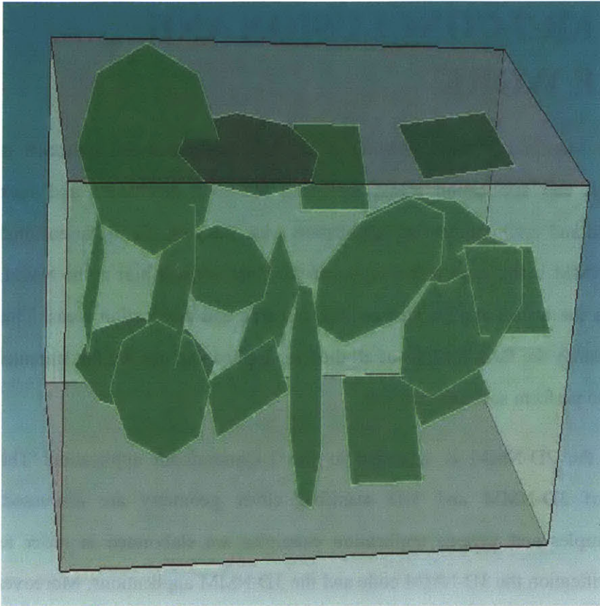
Fig. 6-11: (a) rectangular block model with arbitrary discontinuities; (b) tunnel model with arbitrary discontinuities; (c) cubic model with finite planes inside.
