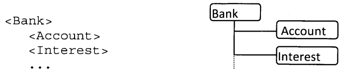
Figure 8. An example of an Association relationship in XML schema (left) and in the content model (right)
