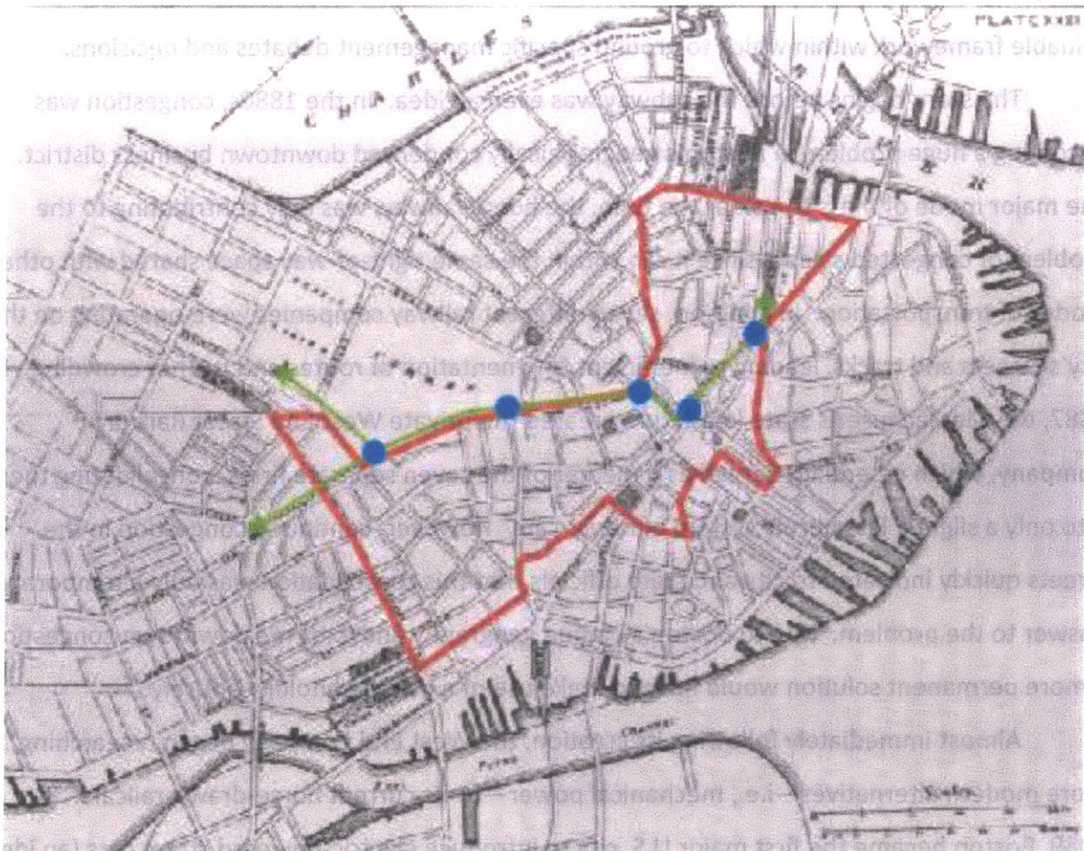
A map of downtown Boston in 1898, showing the congested area (outlined in red) and the new subway (in green). Blue dots represent the original stations, and green triangles show where the subway tracks surfaced to connect to streetcar networks. (Cheape, Moving the Masses [color added by author])
