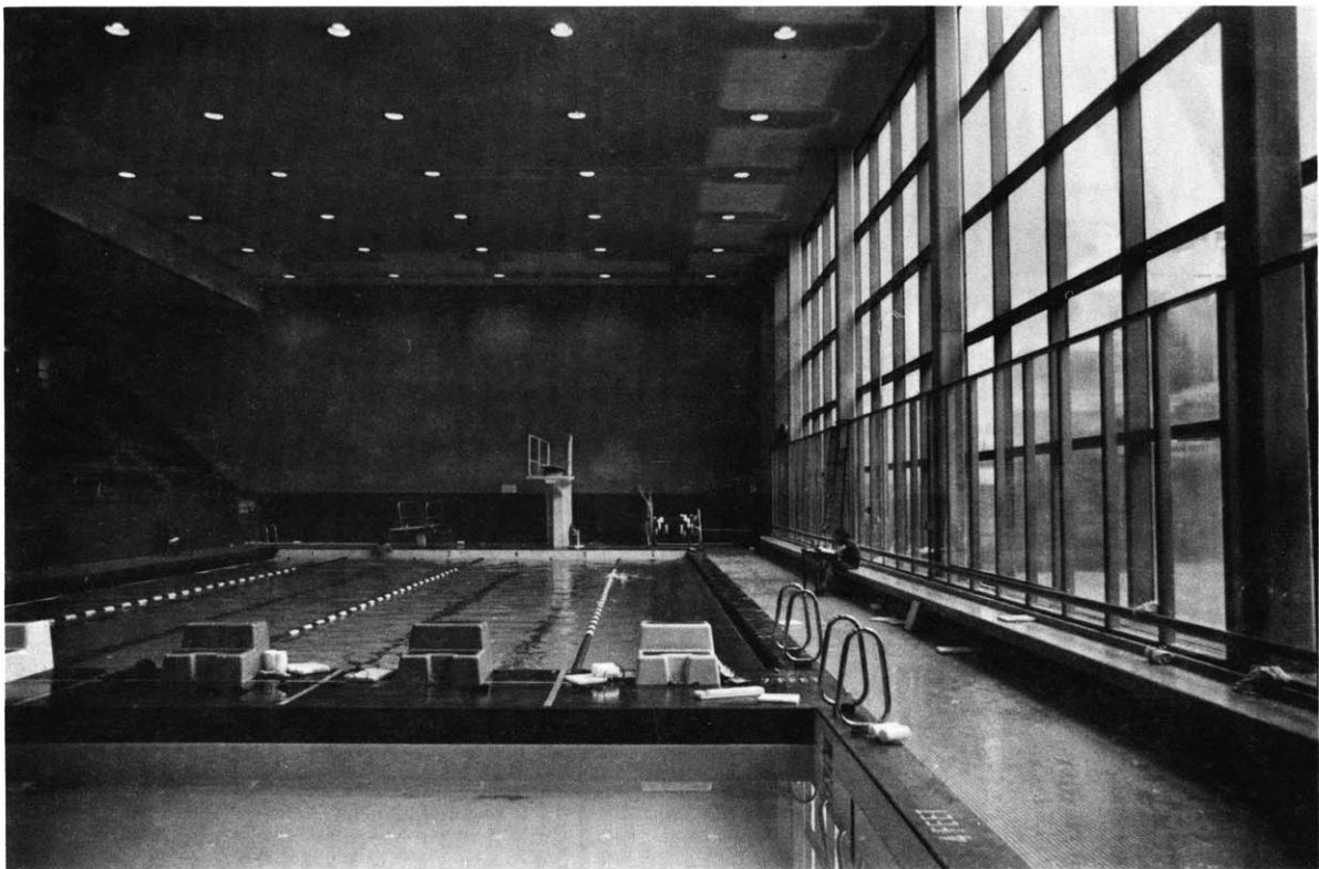
Figure 3.3 MIT's Alumni Pool is lighted by a single south-facing glass wall, but the swimmers experience no visual discomfort because they swim parallel to the window.
