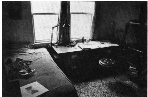
Figure 3.4 A unilaterally-lighted room can have the most extreme contrasts, and can give rise to glare, especially if the windows are small.
