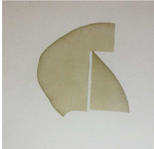
Figure 26: Sample treated at maximum temperature of 255°C showing yellow colour caused by degradation of the material.
