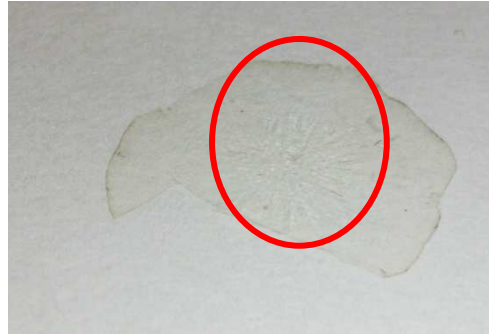
Figure 27: Sample processed with a cooling rate of -10^{\circ}/\text{min} showing imperfections because of fast cooling,
