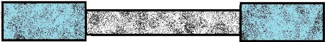
Figure 29: Sketch of an specimen used for tensile test in an INSTRON machine. In white the fluoropolymer, in blue the cardboard tabs and black speckles all over the surface to perform 2D digital image correlation
