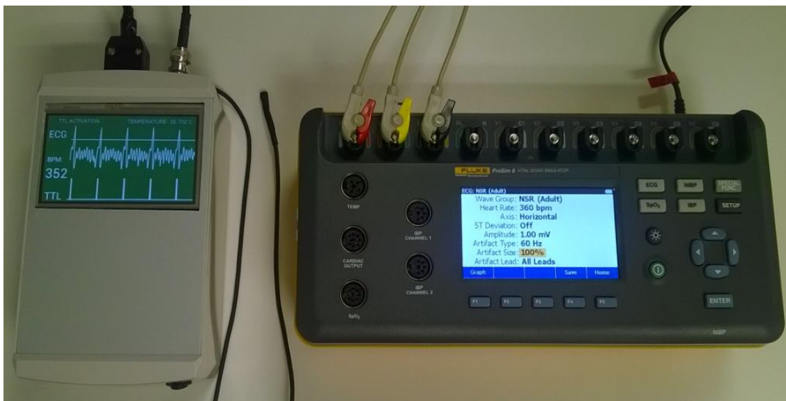
Figure 45. Noise performance: Power line interference (60Hz) at 100%
