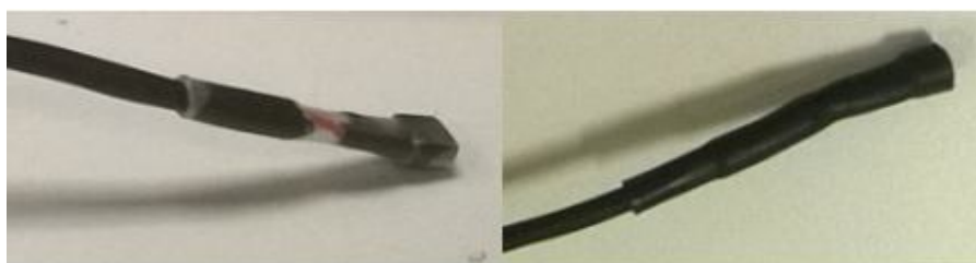
Figure 35. AD22100 sensor at the end of an elongated twisted pair cable as a rectal probe.
