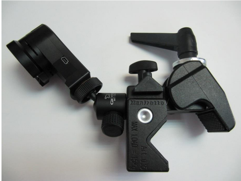
Figure 15: OptiTrack camera attached to Manfrotto Super Clamp.
