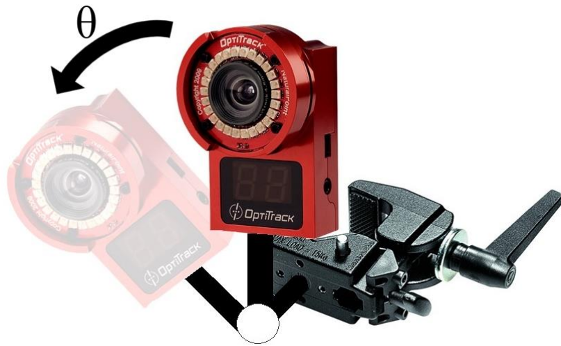
Figure 20: Movement of camera 2 during miscalibration quantification experiment.
