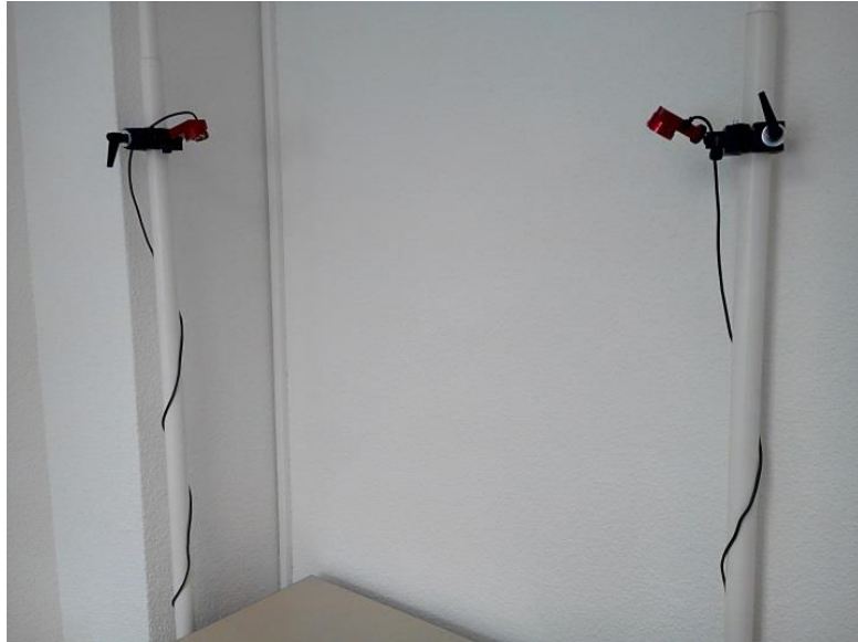
Figure 14: Tracking system composed of two OptiTrack cameras attached to vertical bars (Stolmen posts).
