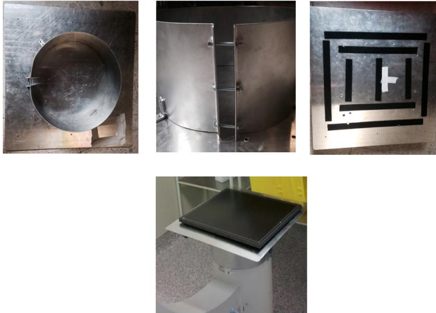
Figure 3. 22 Flat panel's holder. (Top left) Part of the holder that is introduced in the C-arm detector. (Top middle) Screws to adapt the holder to the C-arm detector. (Top right) Part of the holder that is attached to the flat panel. (Bottom) Flat panel with the flat panel using the holder.
