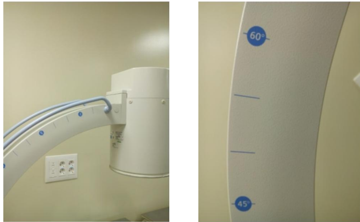
Figure 3. 7 Angular positioning system.
