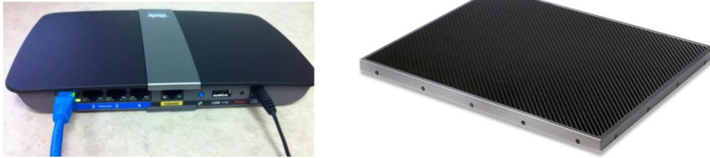
Figure 3. 18 (Left) Wireless Router with Ethernet cable plugged into LAN port. (Right) XRpad 4336 flat panel detector.
