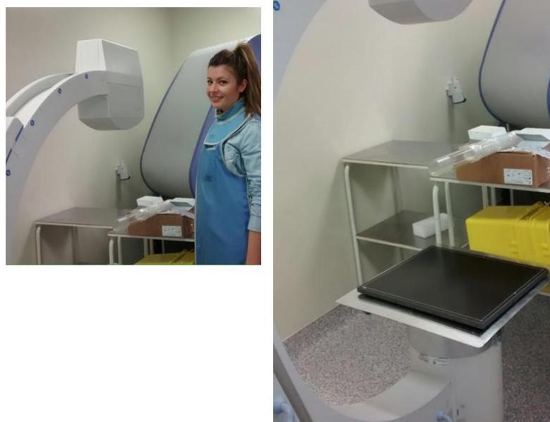
Figure 4. 7 Placement of the phantom in the center of the detector by a plastic tube.
