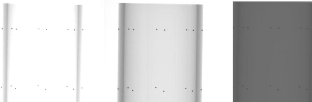
Figure 4.13 Projection image of the calibration phantom obtained with a voltage of 110 keV and an intensity of 3mAs (left), a voltage of 92 keV and an intensity value of 3,6 mAs (middle) and with a voltage of 79 keV and an intensity value (right) of 4.2 mAs.
