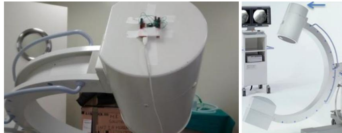
Figure 3. 16 Position of the inclinometer at top of the detector (blue arrow).
