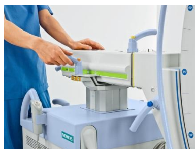
Figure 3. 2 Brakes for the different movement possibilities of the C-arm.
