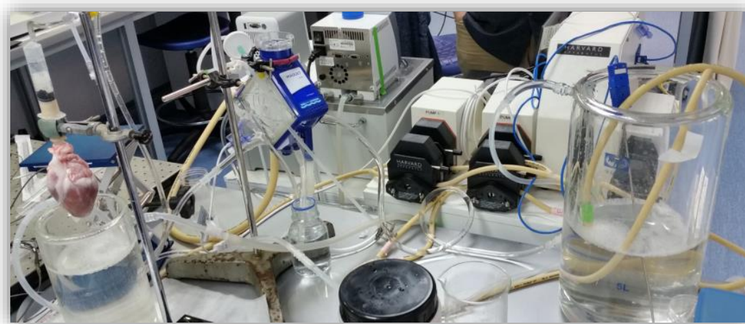
Fig. 21 Langendorff bioreactor set-up at the Unit of Electrophysiology and Arrhythmias within the Laboratory of Bioartificial Organs and Scaffolds.
