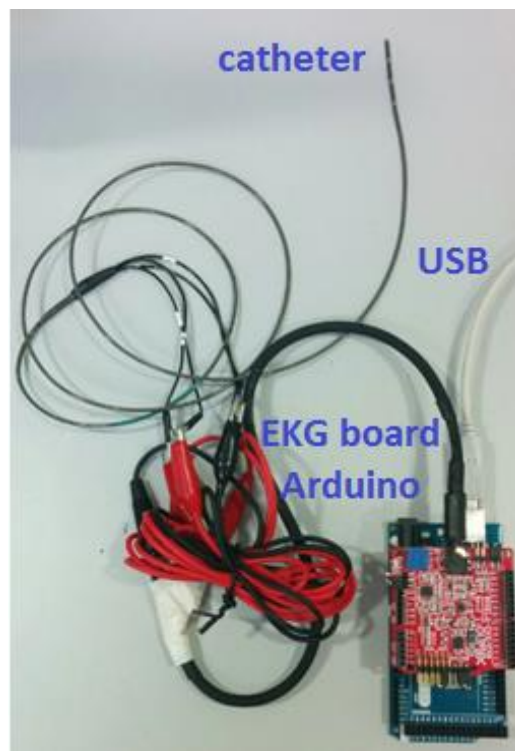
Fig. 23 Registering and analysis platform set-up. A catheter is connected through the jack input to an EKG-EMG board that piggybacks on top of an Arduino Megea256 connected to a PC.
