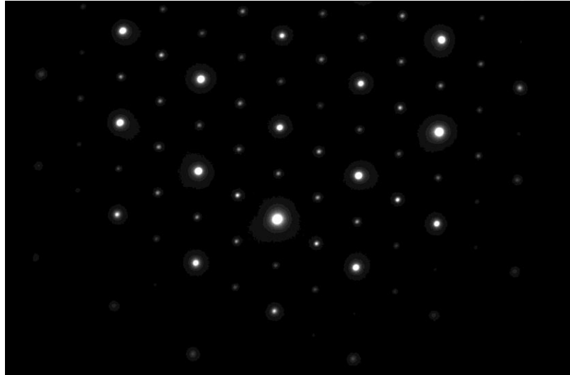
Figure 41. TEM SAD diffraction pattern along the basal zone axis in the WQ sample.
