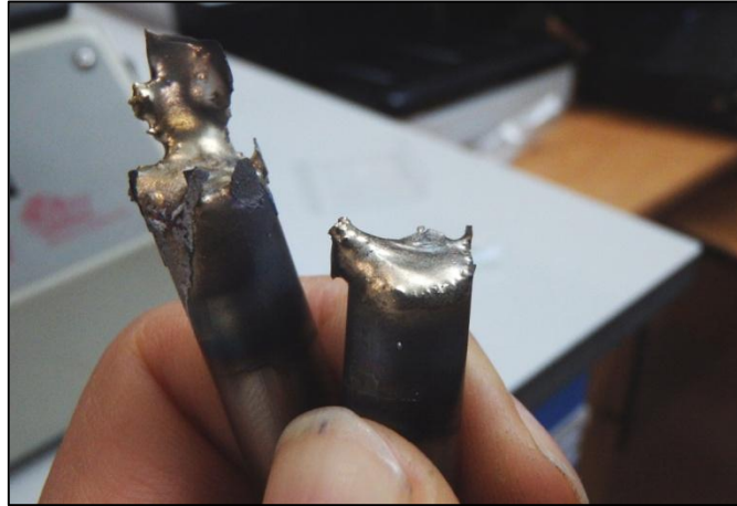
Figure 16. Melted sample due to thermocouple detachment.
