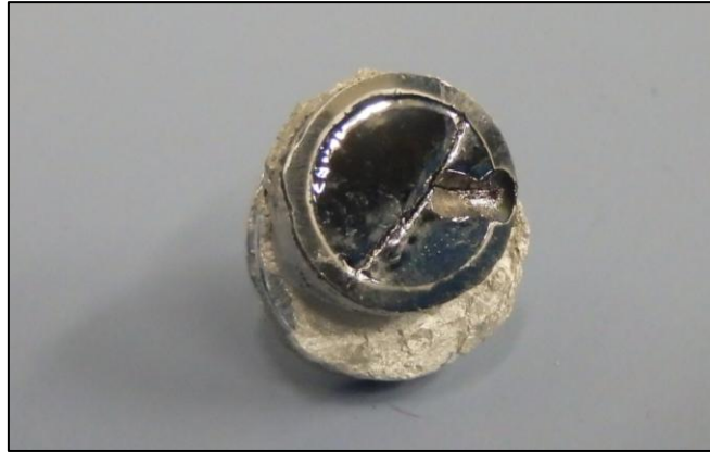
Figure 57. Macroscopic crack in the AWQ sample.
