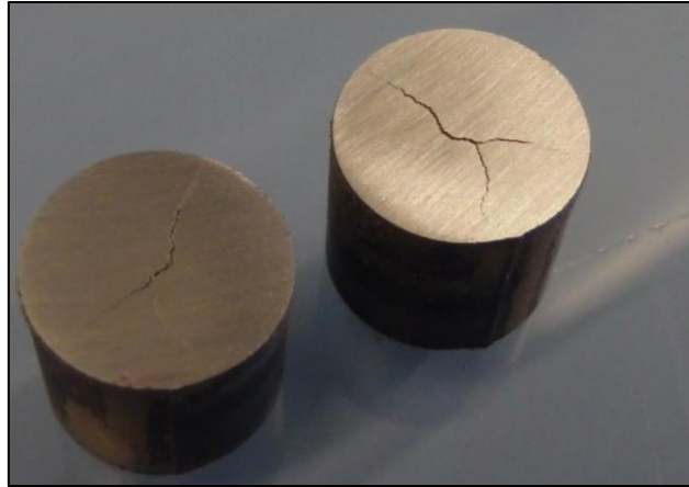
Figure 31. Crack in WQ sample.
