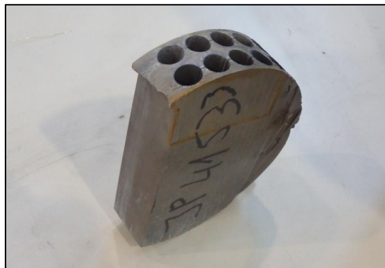
Figure 6. Cast material from which specimens were extracted.
