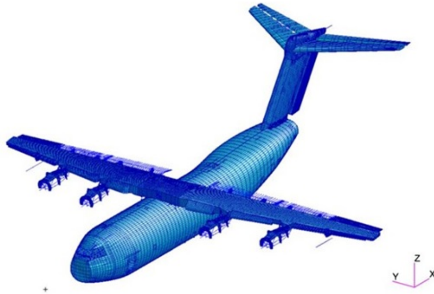
Figure 1.2: A400M Structural model.
