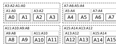
Figure 3: Creating register groups from the physical registers.
