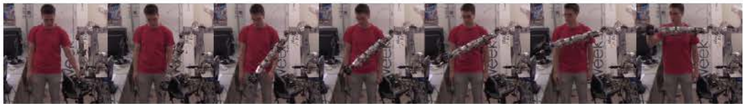
Figure 7.23: Sequence of the movement of the robot arm using a Zero-Friction Zero-Gravity controller. When the user pushes the arm, it moves freely in the direction of the applied force.
