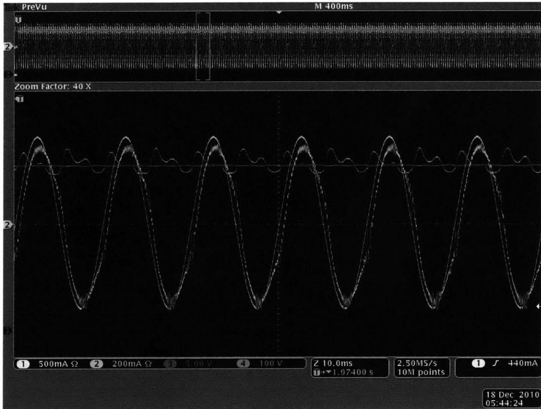
Figure 3.16: The input and output, voltage and current, waveforms for the series-buffer-block prototype converter running into an ac-line, with P_{avg}=100\text{ W} , V_{PV}=32\text{ V} , V_{buf}\approx 170\text{ V} , V_{ac}=240\text{ V}_{\text{rms}} . The waveforms are CH1: Input Current, CH2: Output Current, CH3: Input Voltage, CH4: Output Voltage.
