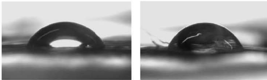
FIGURE 3.12: Contact angle between E-glass fabric and a drop of corn syrup fluid (80%).
