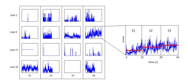
Figure 69. Four random users' performance results in the four experiments. The x axis is the time and the y axis is the genuine score. The red lines are the scores mean for each time slot ( $\mu' \in R$ ).
