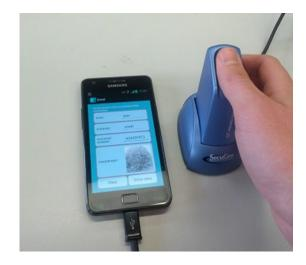
Figure 3. Biometric fingerprint obtained with a fingerprint sensor connected to a smartphone
