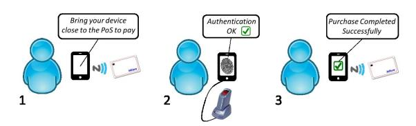
Figure 56. Example of app's use. The communication starts in 1, then in 2 is the biometric recognition. In 3 the fictitious payment is made. The smartcard acts as the PoS and communicates with the smartphone through NFC
