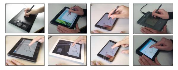
Figure 13. Devices used during the evaluation. In the first row are the stylus-based devices. From left to right: Wacom Intuos 4, Asus Eee Pc T101 MT, Samsung Galaxy Note and Wacom STU-500. The fingertip-based devices are in the second row. From left to right: Blackberry Playbook, Apple iPad 2, Samsung Galaxy Note and Samsung Galaxy Tab.
