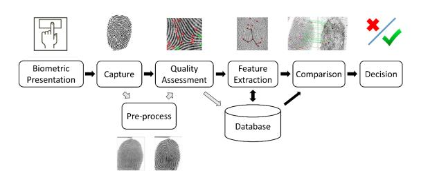
Figure 2. General phases of the biometric recognition process
