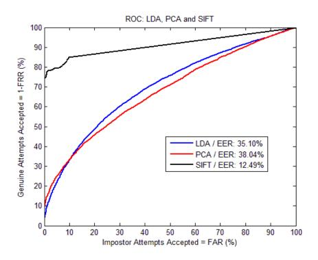
Figure 67. LDA, PCA and SIFT ROC curves including the EER
