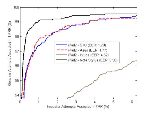
Figure 19. iPad2 template vs. Stylus based devices
