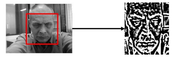
Figure 66. Image before and after the Pre-processing. The red square is the bounding box
