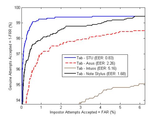
Figure 20. Tab template vs. Stylus based devices
