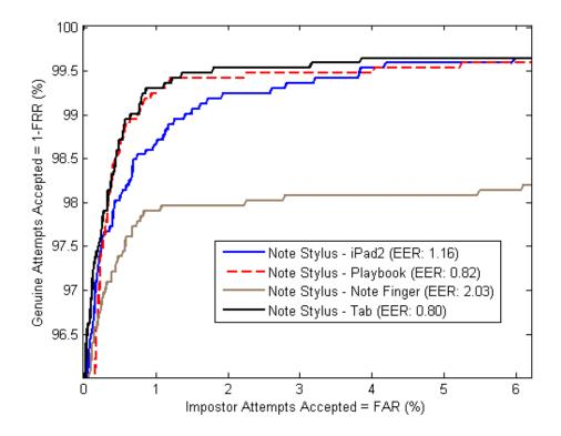
Figure 17. Note-Stylus enrolment vs. Fingertip-based devices
