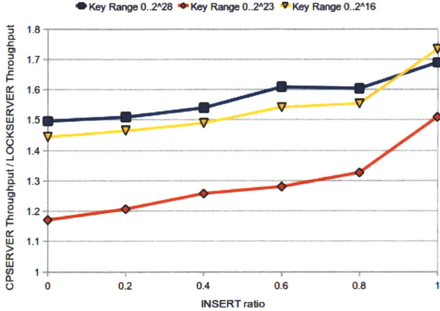
Figure 6-5: CPSERVER throughput vs LOCKSERVER throughput
