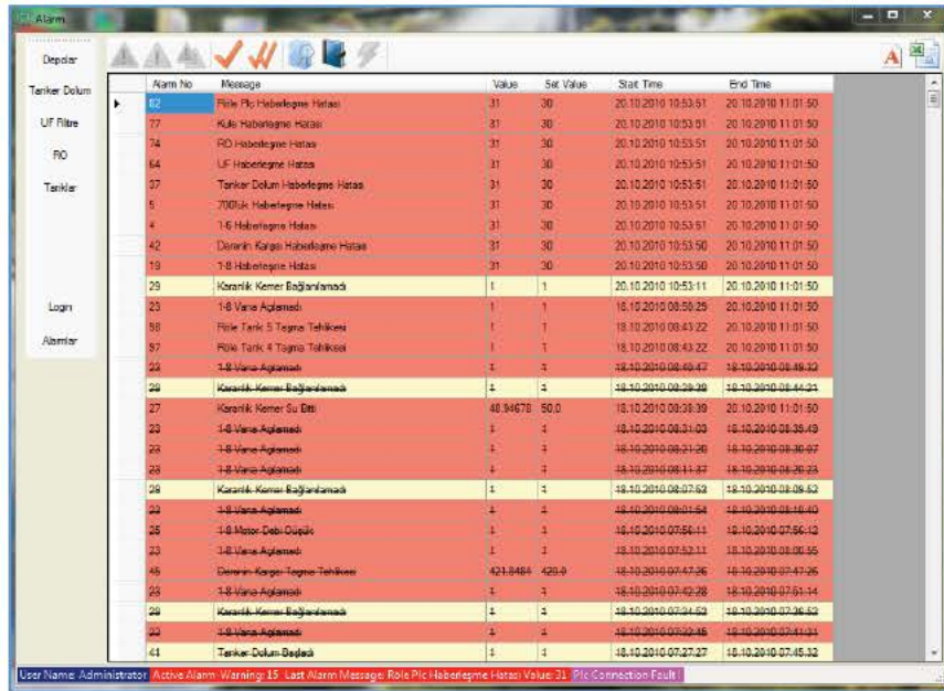
Annex Fig. A-21 An implementation of the Lists pattern: Alarm lists displaying the chronological order of alarms in a CAS data logger interface [22]
