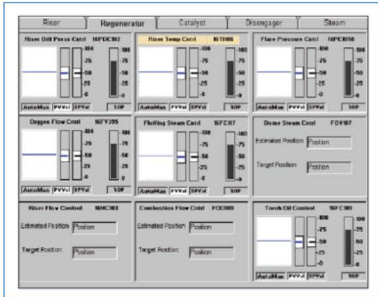
Annex Fig. A-7 An implementation of the Secondary level pattern: ASM-style secondary level display [107]
