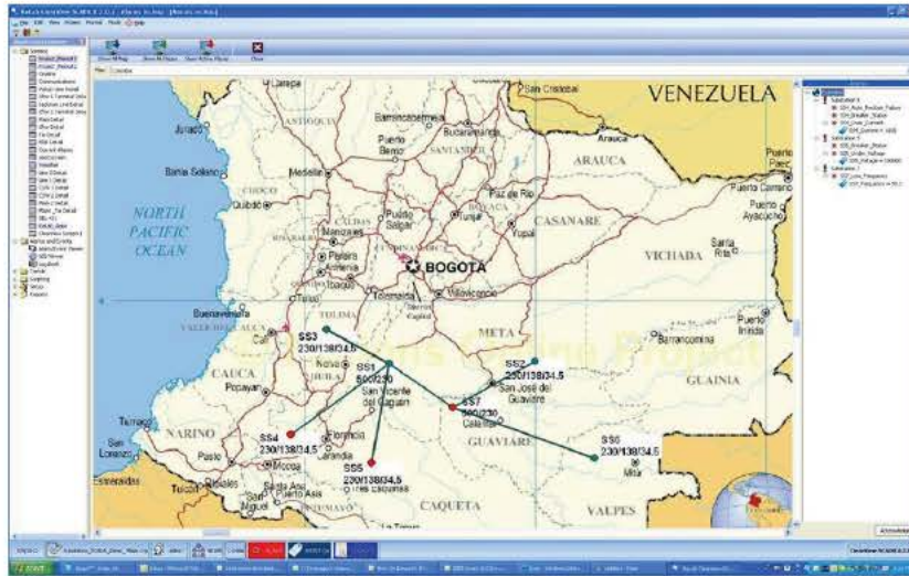
Annex Fig. A-29 An implementation of the Maps pattern: ClearView SCADA Geographical Information System enables visualization of alarm information organized geographically with drill down and display capability into the assets to obtain detailed information about the alarm or event [29]
