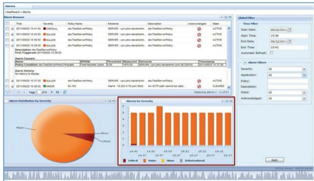
Annex Fig. A-34 An implementation of the Bar charts pattern: IrisView system alarm dashboard which gives the operator a view of any alarms associated with the elements they are responsible for (see a bar chart for alarm activation rates per device framed in red) [65]
