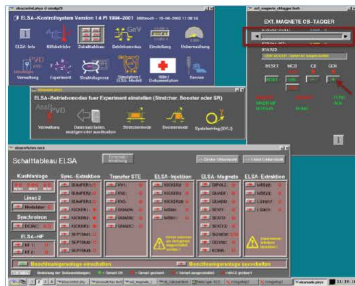
Annex Fig. A-41 An implementation of the Direct manipulation pattern: Use of sliders (framed in red) and buttons (pointed by the arrow) to allow the human operator to provide inputs to the ELSA control system interface [42]
