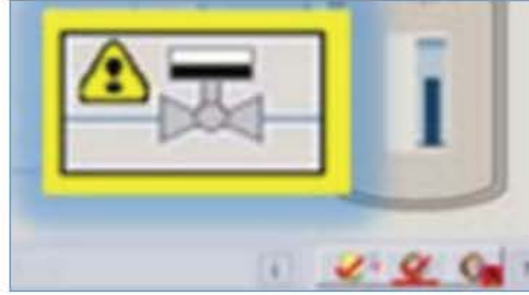
Annex Fig. A-25 An implementation of the Flashing pattern: Top priority alarm stand out by using flashing in DeltaV control system [43]
