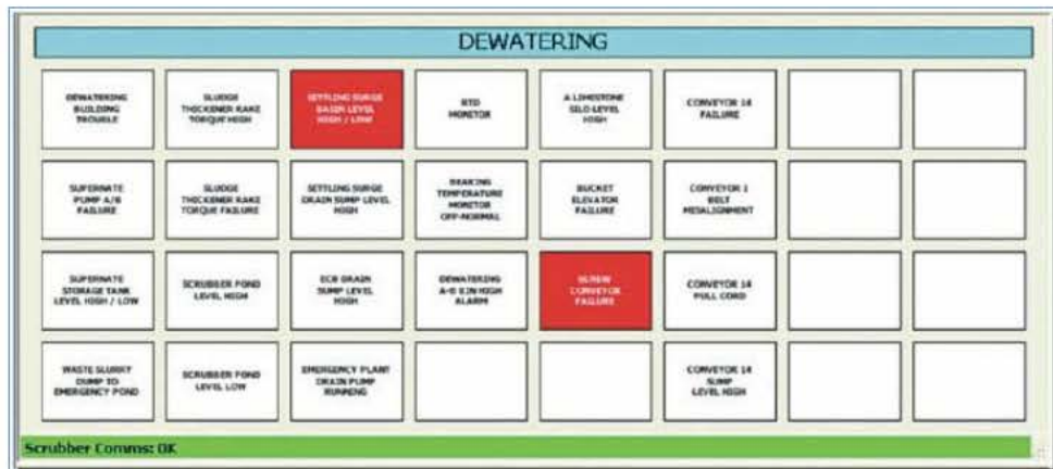
Annex Fig. A-11 An implementation of the Tiled layout pattern: Y-Plant Alert Alarm Annunciator System [146]
