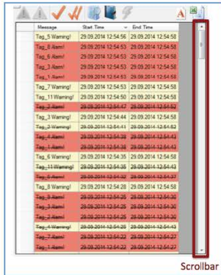
Annex Fig. A-53 An implementation of the Scrolling pattern: Alarm list with scroll bar vertical enabled from a SCADA system interface [113]
