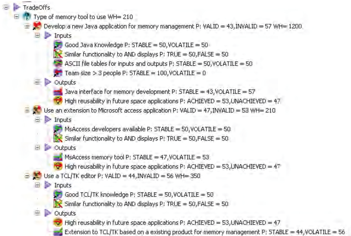
Figure 6-21: Tree view probability propagation once a fact for an input is set
