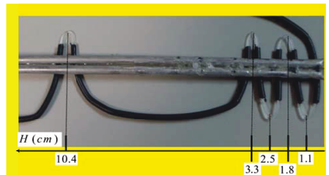
Fig. (5). Photo of a fiber-optic sensor prototype manufactured for fuel level measurements.
