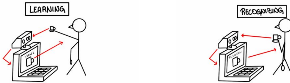
Figure 4.1: OCULAR working modes: learning (left) and recognizing (right). The learning mode is triggered when the user stretches his/her arm towards the robot. The recognizing mode is triggered when the user pulls his/her arm towards his/her chest. This is the default mode.
