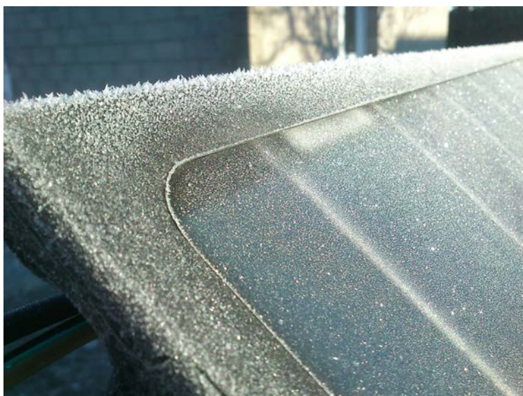
Figure 6.25: Morning frost over modules' frontal surface.
