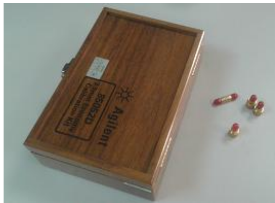
Figure 3.10. Network Analyzer Agilent 8703B Calibration kit.
