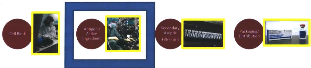
Figure 6-2 Typical Manufacturing Flow for Biotech/Vaccine Production
