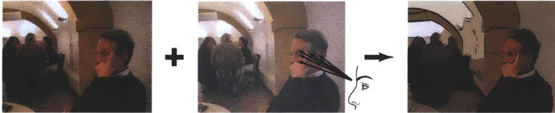
Figure 2-5: A model of attention can be used for stylization and abstraction of images as demonstrated in the work of [DeCarlo and Santella, 2002]. An eye tracker determines where people look in an image. The data is used to drive the level of detail at each location in the non photorealistic rendering of the image: more details where people looked and less elsewhere. Images reprinted with permission from DeCarlo and Santella [2002].
