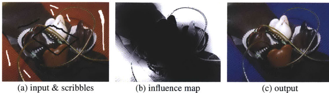
Figure 3-7: Fast scribble interpolation using the Bilateral Grid. The user paints scribbles over the input (a). Our algorithm extracts an influence map (b), which is used to adjust the input hue and produce the output (c). The entire 2 megapixel image is updated at 20 Hz. Memory usage was about 62 kB for s_s = 256 and s_r = 0.05 .
