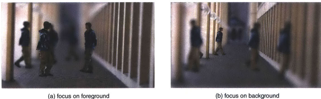
Figure 4-8: Compositing and depth of field manipulation. We replicated the character from the original video, composited multiple copies with perspective, and added defocus blur.
