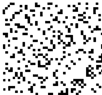
Figure 6.4. An adjacency matrix of a sparse, well-connected graph example obtained using the approach described in Section 6.5.2: The weights of this graph lie in the range [0, 1] , the black points represent edges with nonzero weight, and the white points denote absence of edges. The (weighted) degree of each node is 8, the average number of nonzero (weighted) edges per node is 8.4, the second-smallest eigenvalue of the Laplacian is 4, and the weighted diameter is 3.
