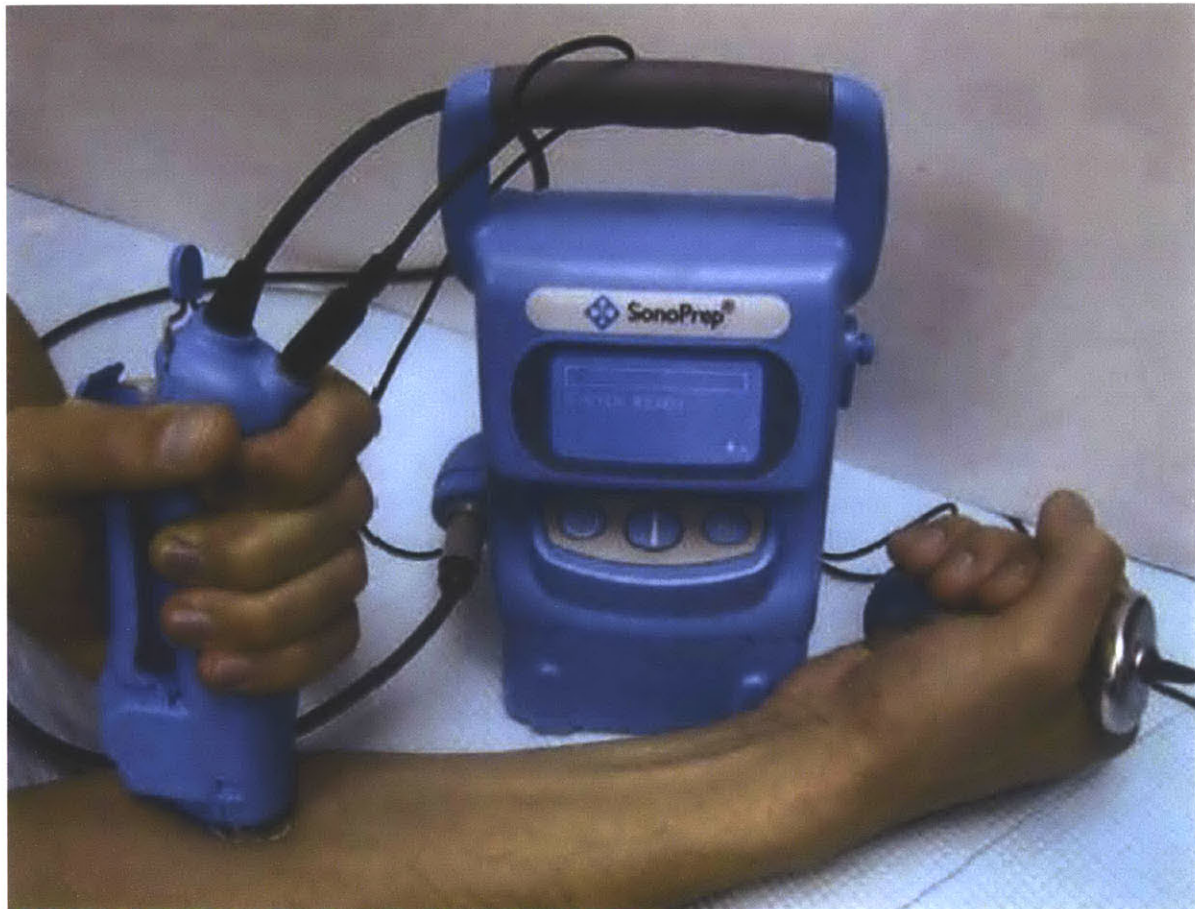
Figure 1-7. Low-frequency ultrasound treatment in a clinical setting with the SonoPrep® device (Echo Therapeutics, Franklin, MA). The patient holds a conductive polymer hand-piece and the device automatically stops when the skin impedance is decreased to the desired treatment level. Usual treatment times are on the order of 10 seconds.
